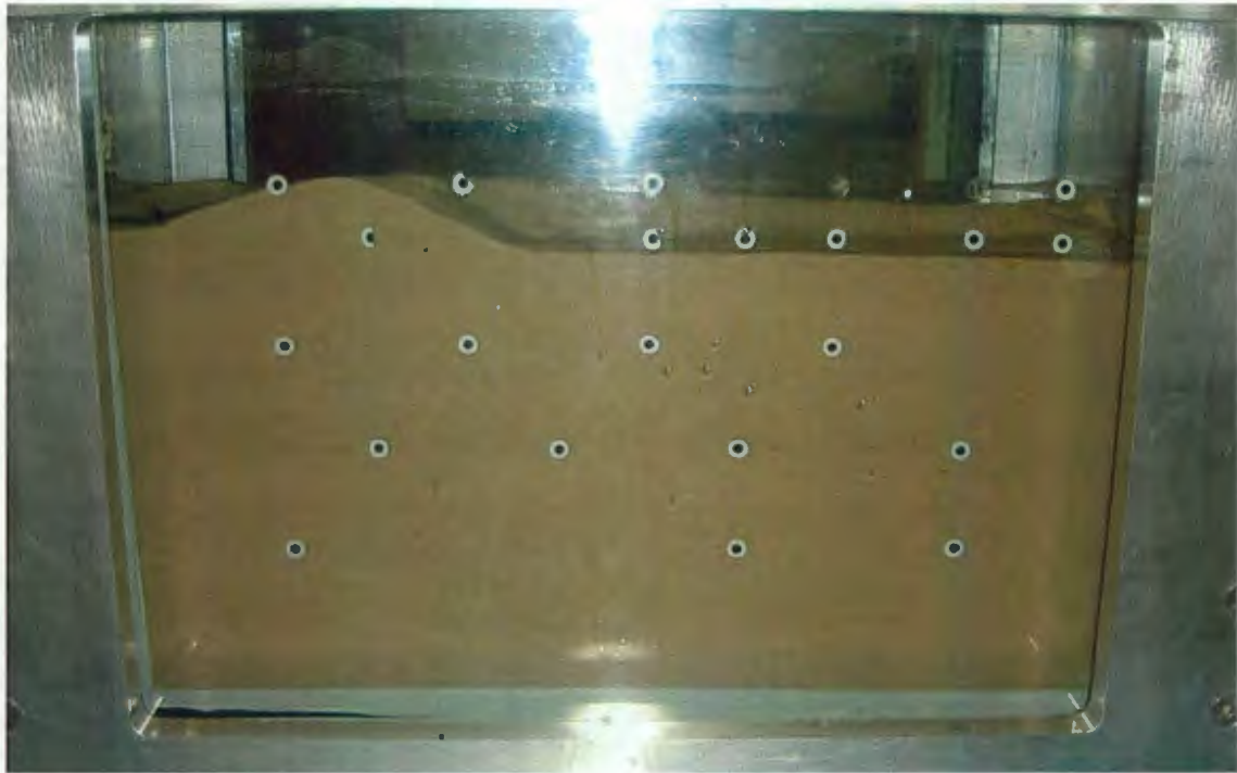
Figure A. 26 Side view of gouge shape for test P08
