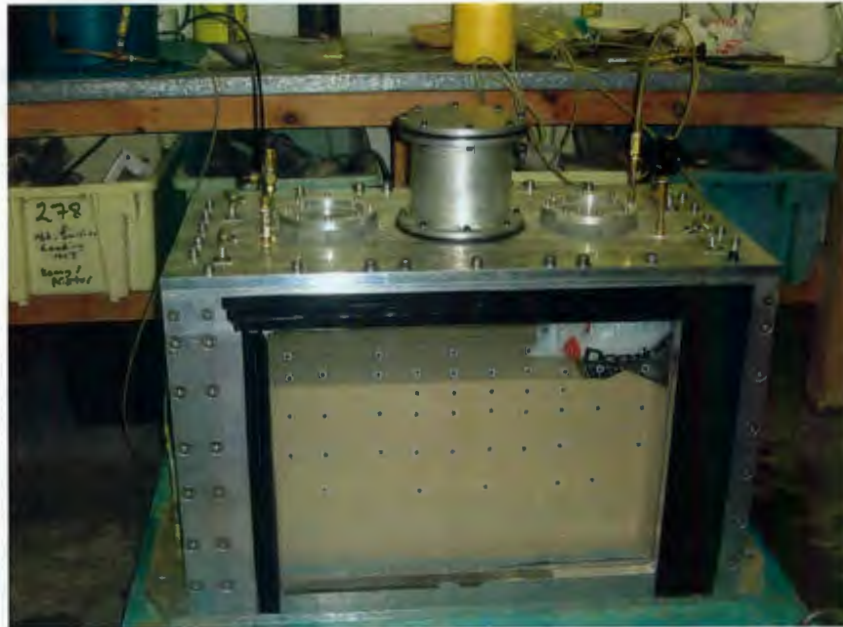
Figure 4-3 Configuration of the sample container during saturation process
