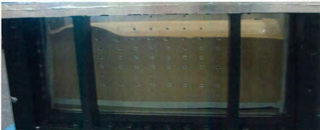
Figure A. 24 Side view of gouge shape for test P07
