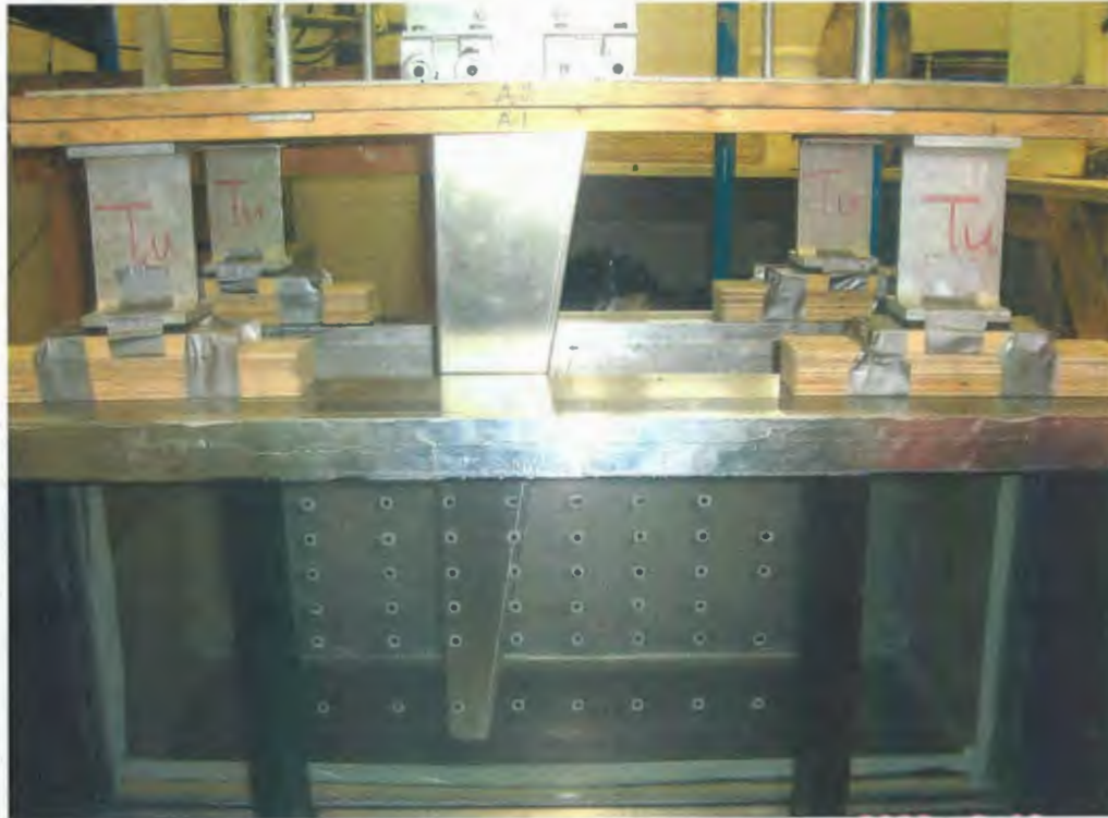
Figure 4-1 Setup of the sand raining tool
