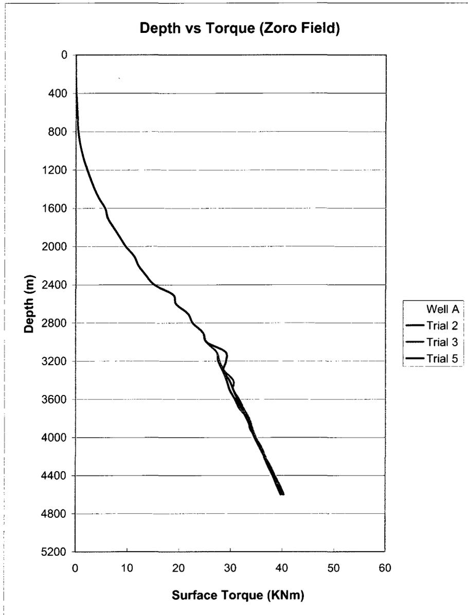
Figure 6.10: Torque Profile for Wells in Zoro Field
