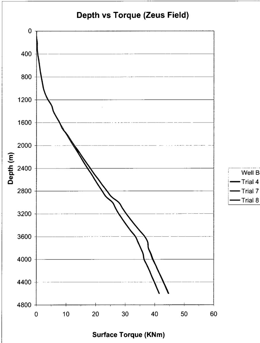
Figure 6.22: Torque Profile for Wells in Zeus Field
