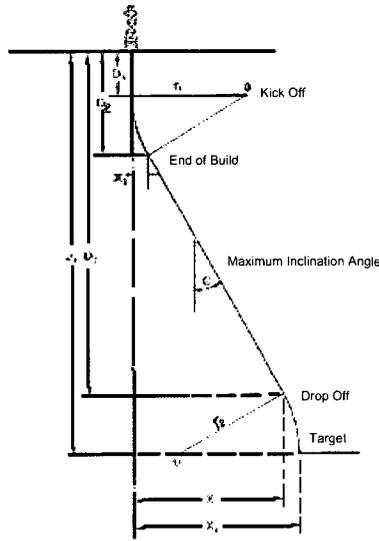
Figure 2: A2 - Build, Hold & Drop Trajectory (Profile 1)
