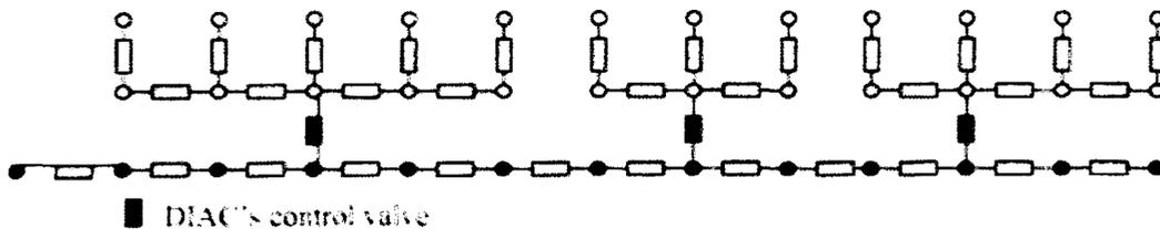
Figure 3.2: *NETool*<sup>™</sup> Node Configuration for DSAV Completion
