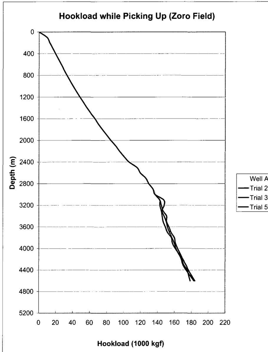
Figure 6.12: Hookload While Picking Up Profile for Wells in Zoro Field
