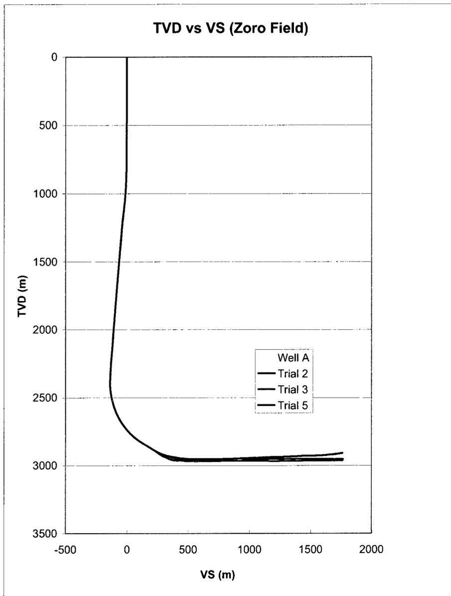
Figure 6.6: Vertical Profile of all Wells in Zoro Field
