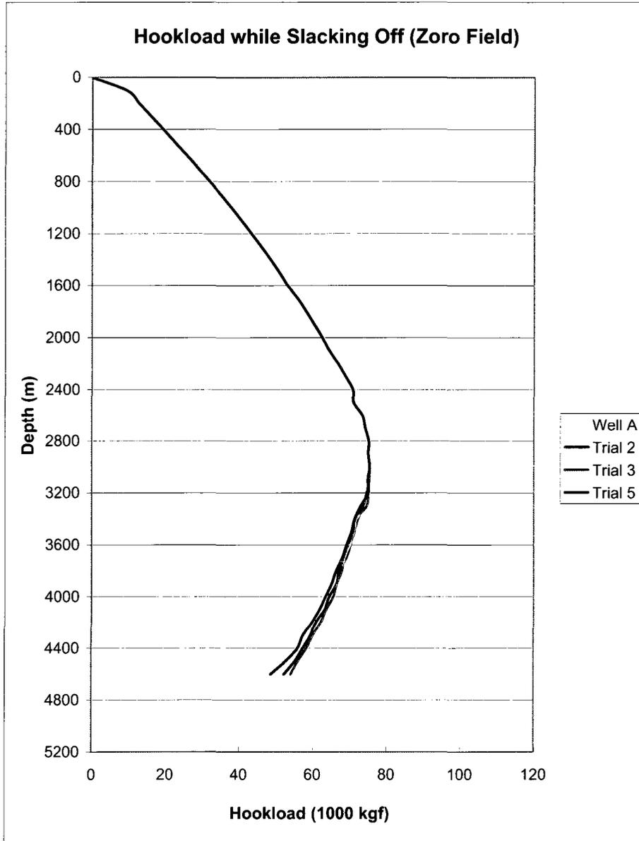
Figure 6.13: Hookload While Slacking Off Profile for Wells in Zoro Field
