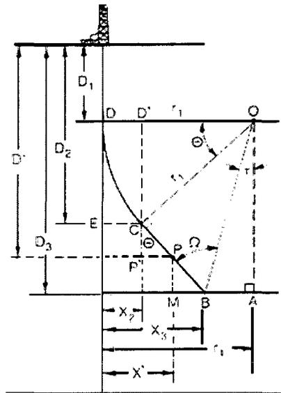
Figure 1: A1 - Build and Hold Trajectory
