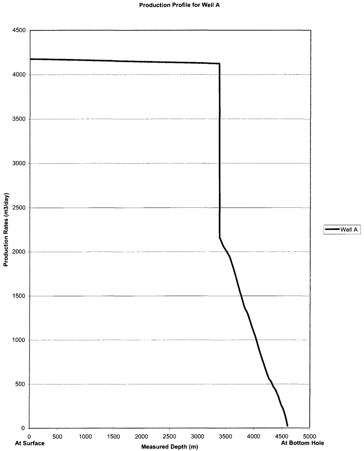
Figure 6.1: Production Rate Profile for Well A
