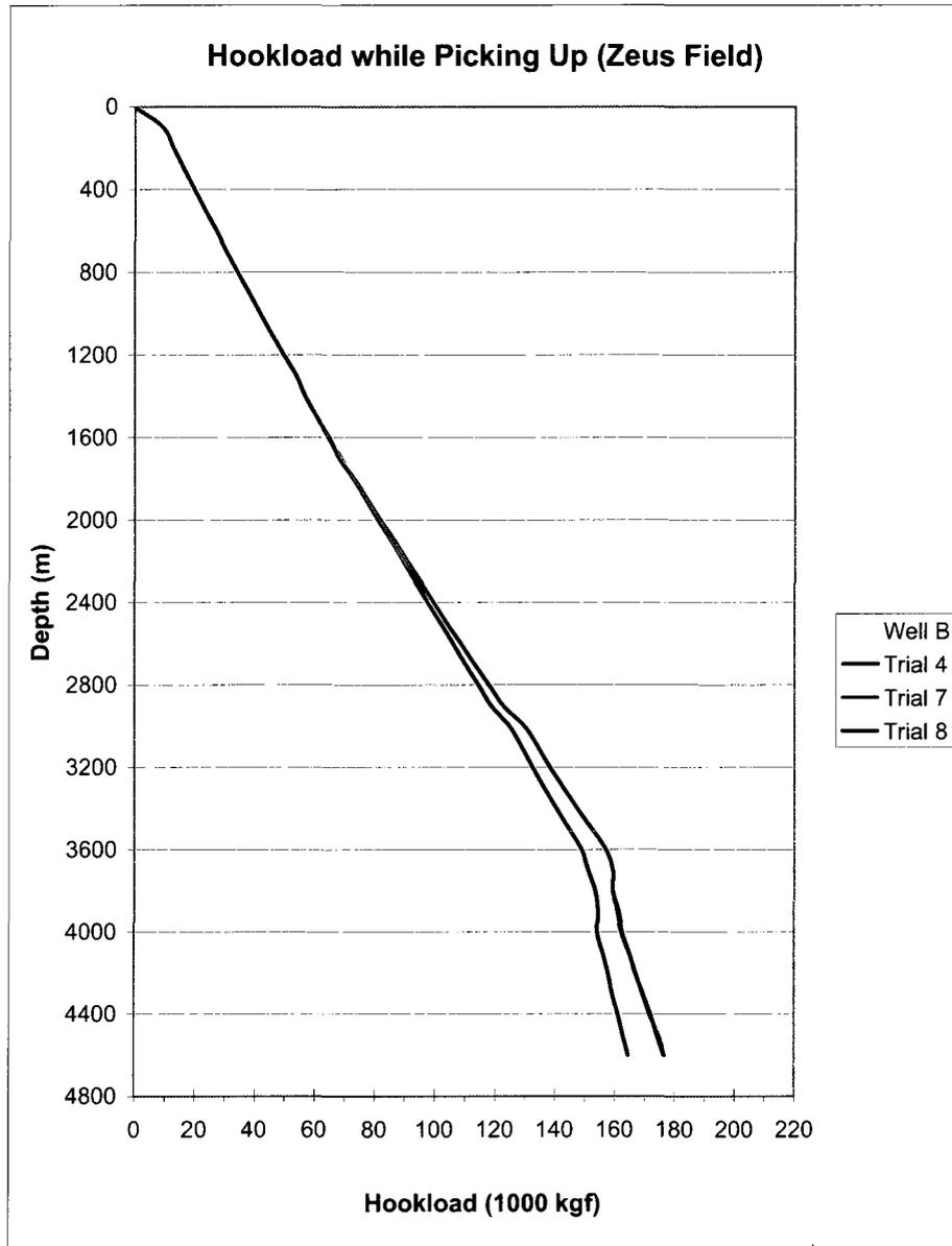
Figure 6.24: Hookload While Picking Up Profile for Wells in Zeus Field
