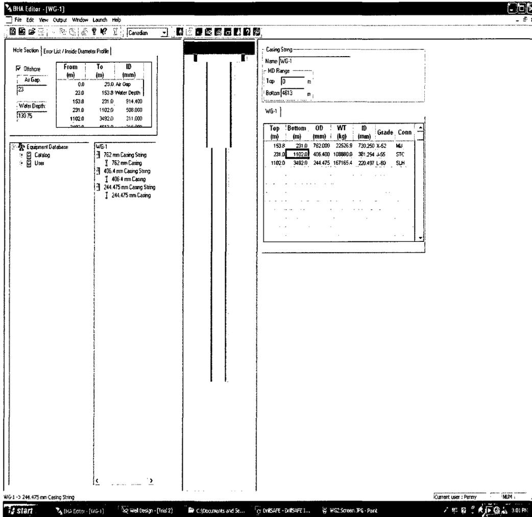
Figure 6.4: Well Geometry and Casing Details for Zoro Field
