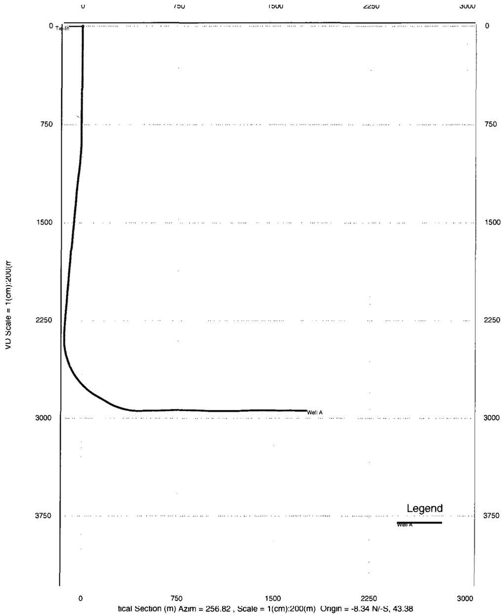
Figure 6.2: Vertical Profile of Well A
