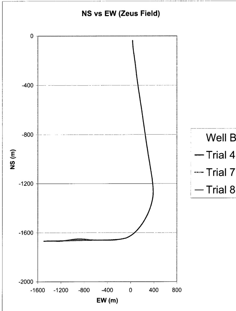
Figure 6.20: Horizontal Profile of all Wells in Zeus Field
