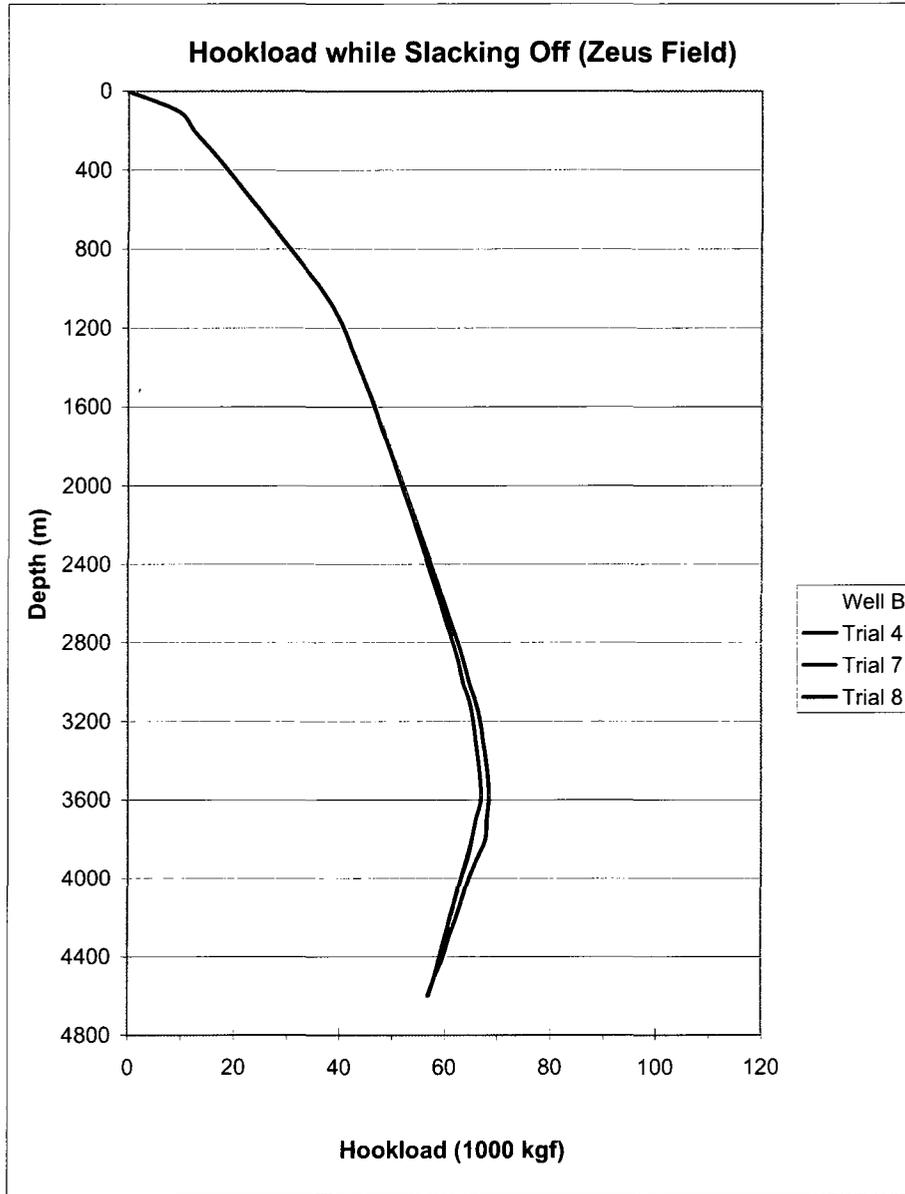
Figure 6.25: Hookload While Slacking Off Profile for Wells in Zeus Field
