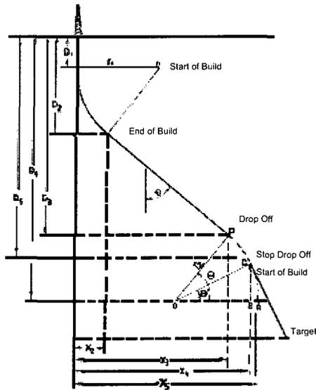
Figure 3: A3 - Build, Hold & Drop Trajectory (Profile 2)
