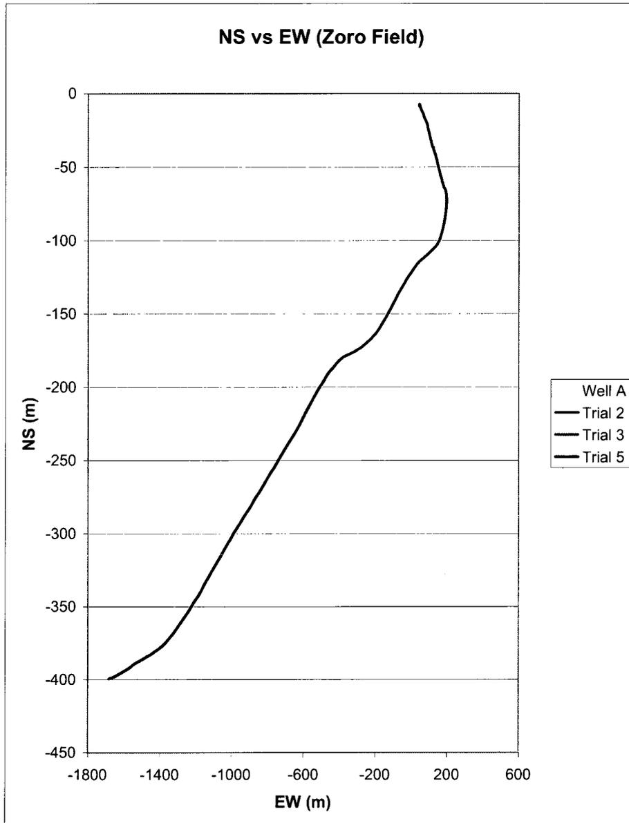
Figure 6.7: Horizontal Profile for all Wells in Zoro Field
