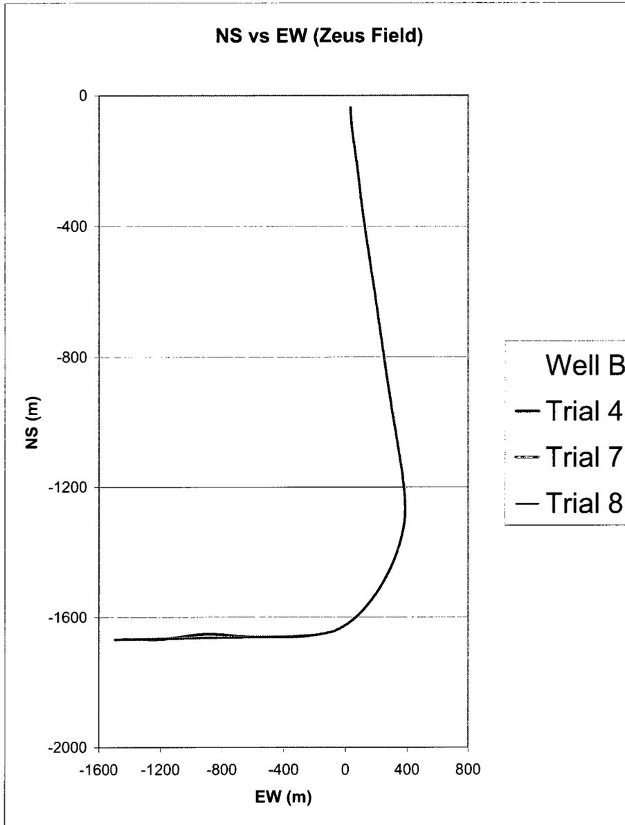
Figure 6.20: Horizontal Profile of all Wells in Zeus Field
