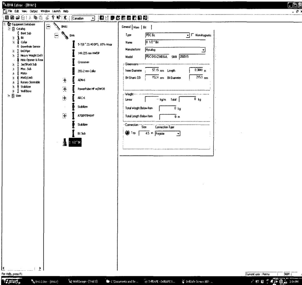
Figure 4.2: PowerPlan<sup>®</sup> BHA Editor Bit Assembly Screen
