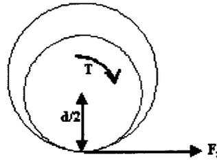
Figure 5: B2 - Pipe Lying in Bottom of Wellbore
