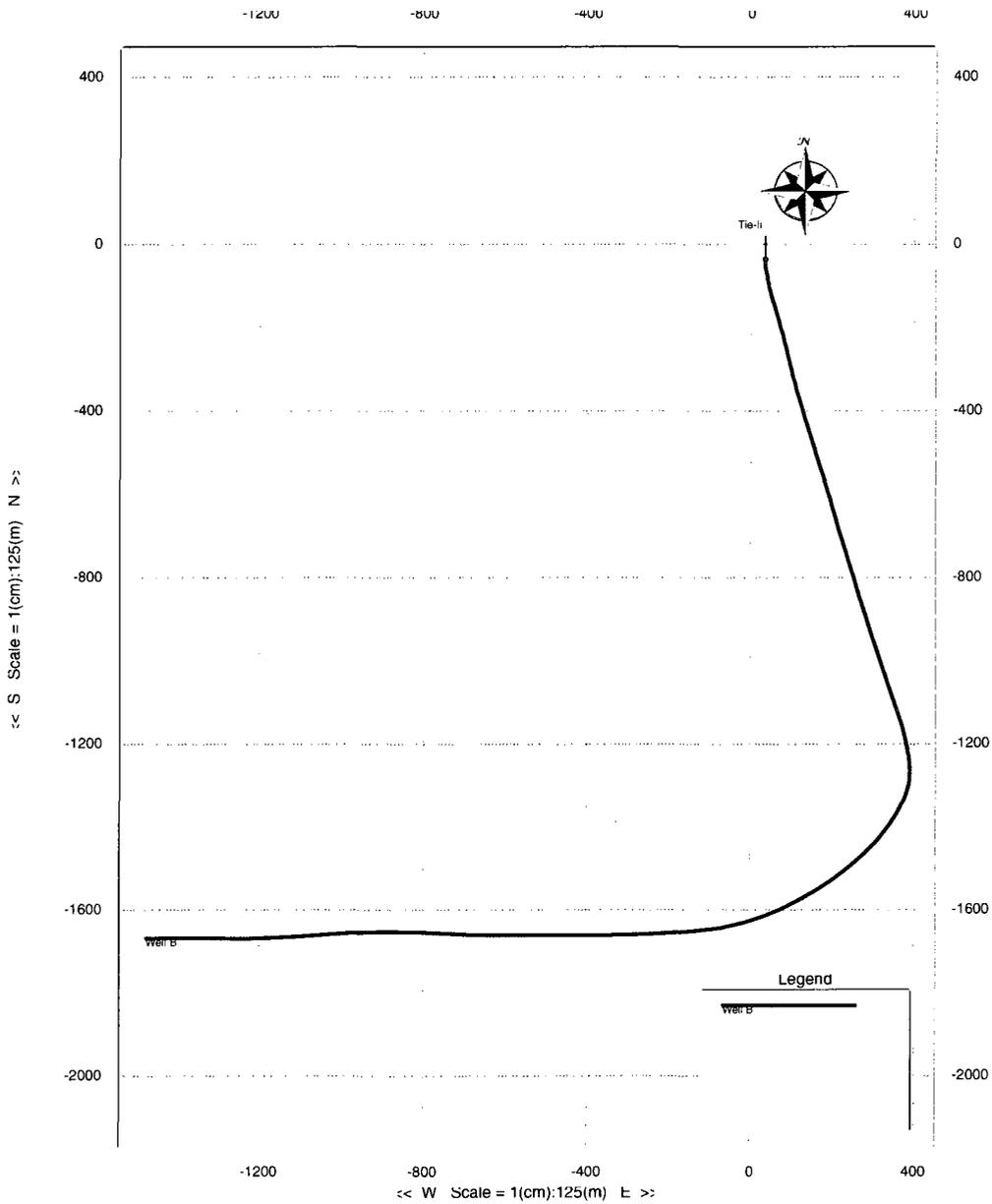
Figure 6.16: Horizontal Profile of Well B
