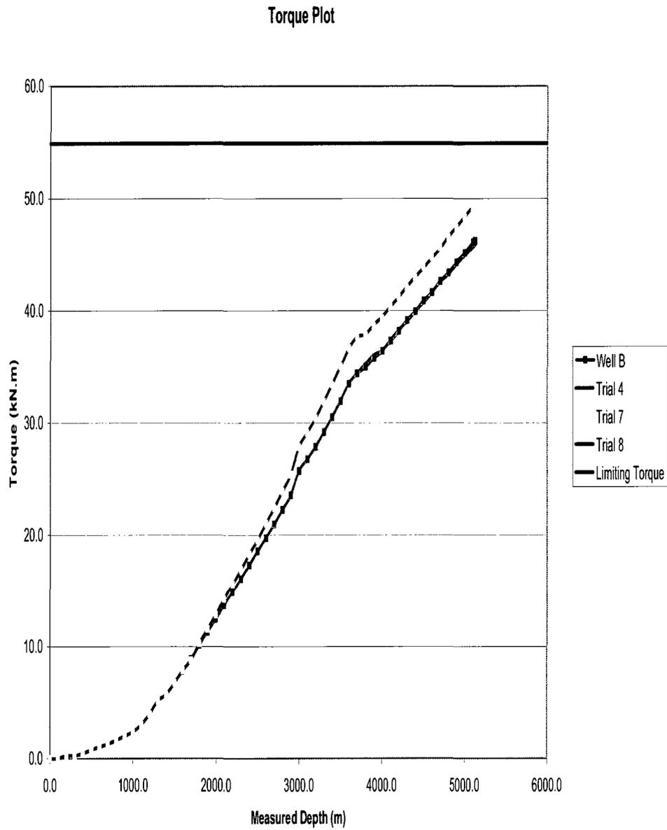
Figure 7.9: Torque Plot for Case Study 2
