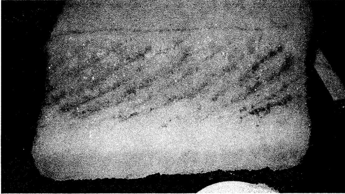
Figure 3-6: Ice sample after underwater milling tests
