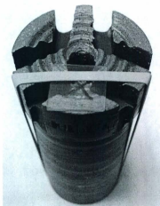
Figure 21. Glass plate on top of full face bit
