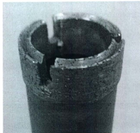
Figure 17. Impregnated diamond coring bit
