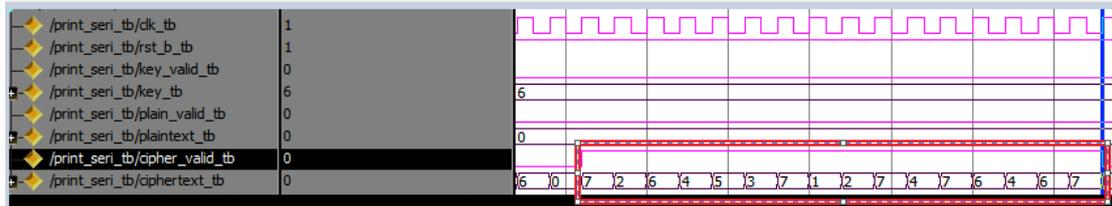
Figure 4.12 Simulation Result of the Serialized Design of PRINTcipher
