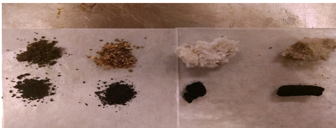
Figure 1.3. Top row, dry feedstocks left to right: sewage sludge, chicken litter, gable, egg carton. Resulting char directly below original feedstocks.
