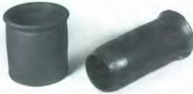
Figure 35: Building Materials: Unglazed thimble and drain pipe (Zug 1986: 353).
