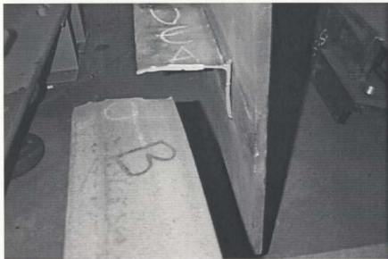
Figure 5-2 Failure of Angle in Tension-type Tearing
