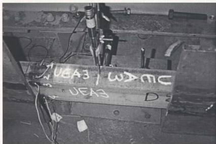
Figure 4-8 Measurement Devices on Angle Specimens
