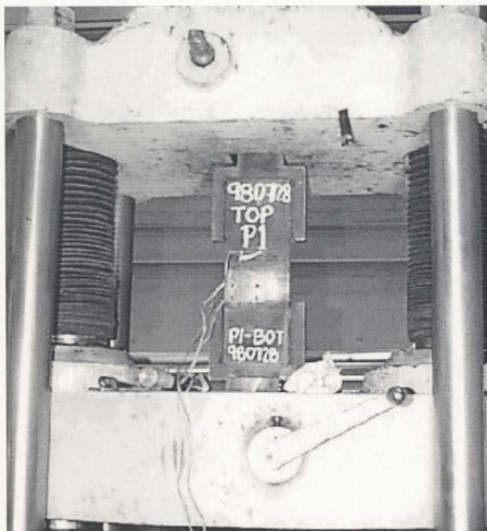
Figure 4-4 Test on Tinius-Olsen UTM
