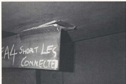
Figure 5-3 Failure of Weld under Bending and Shear
