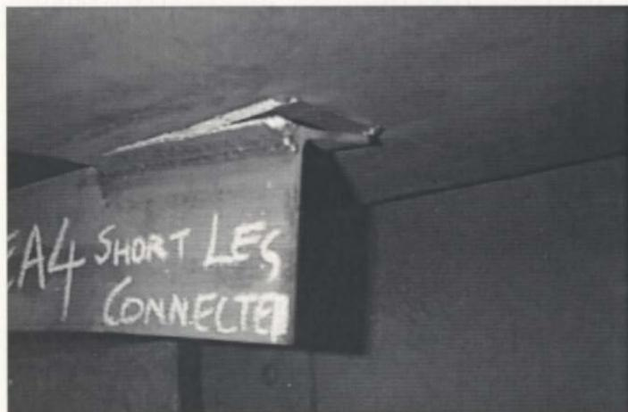
Figure 5-3 Failure of Weld under Bending and Shear
