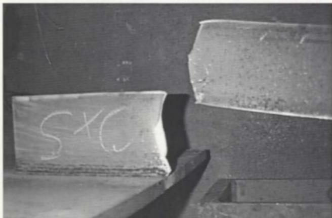
Figure E-2 Failure of Specimen P120-S
