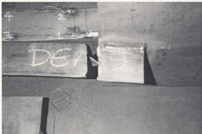
Figure F-3 Failure of Specimen DEA5
