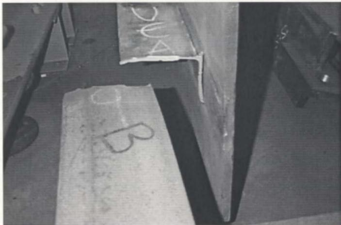
Figure 5-2 Failure of Angle in Tension-type Tearing
