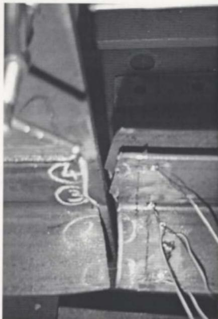
Figure F-1 Failure of Specimen DEA2
