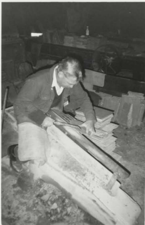
Plate 47. Slater from Holme's Academy or Armory , dated 1688 (above), Craftsman at the Welsh Slate Museum: trimming (below).
