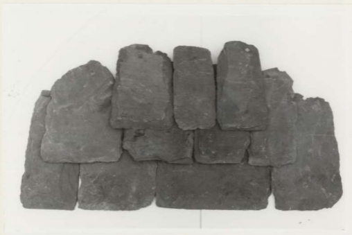
Plate 53. Roof slate terminology (above), example of overlapping courses (below).
