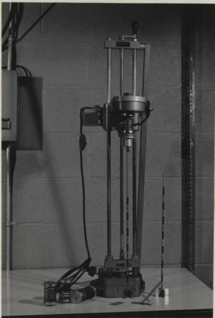
FIG. 38.- PHOTOGRAPH OF THE MODIFIED VANE SHEAR APPARATUS
