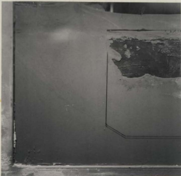
FIG. 72.- PHOTOGRAPHS SHOWING THE SOIL FAILURE IN FRONT OF THE 2" WIDE MODEL WITH CHAMFERED TOE
