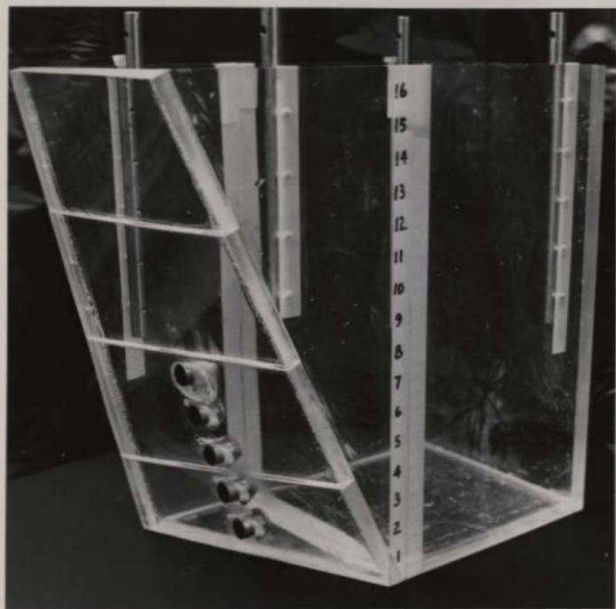
FIG. 34. - PHOTOGRAPH OF THE MODEL M<sub>3</sub> WITH A TWISTED AND INCLINED FRONT FACE.
