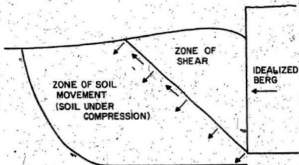
FIG. 76.- CONCEPTUAL SOIL MOVEMENT IN FRONT OF THE IDEALIZED BERG
