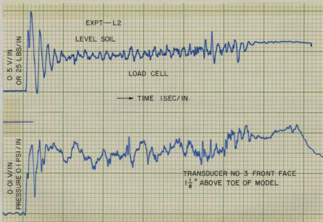
FIG. 45. RAW DATA OF TOTAL PULL AND PRESSURE FROM THE EXPERIMENT IN A LEVEL SOIL SURFACE
