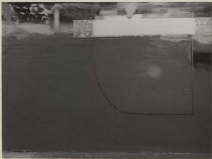
FIG. 74. - PHOTOGRAPH SHOWING THE SOIL FAILURE IN FRONT OF THE MODEL WITH A ROUNDED FRONT
