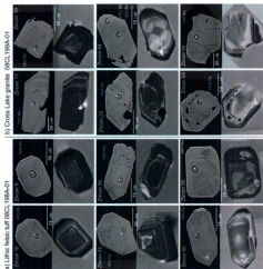
Figure 2.16: Representative zircon grains in both backscatter electron (BSE) and cathodoluminescence (CL) images for two samples from Middle Head: a) foliated crystal-lithic felsic tuff (08CL198A-03); and b) foliated Cross Lake granite (08CL199A-03). Analytical SHRIMP spots can be seen in the grains.
