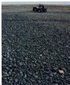
Figure 3.27 Quickbird satellite image of Clyde River, August 21, 2005. Letter A refers to photo location. North of the airport, a large glaciofluvial terrace on either side of the Clyde River contains abundant cobble-sized gravel. Depending on the quantity of material, this site could provide the community with much needed granular aggregate for building pads and other infrastructure demands (photo T. Bell, July 2007).
