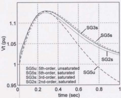
Figure 4.8 Effect of saturation on SG transients, Case #1
