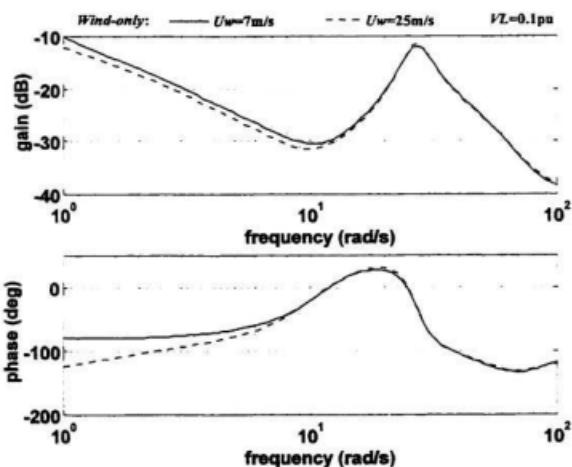
Figure C.3 Bode diagram of *wind-only* configuration.
