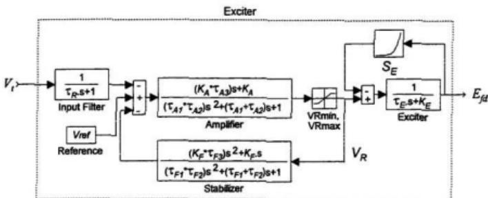
Figure 3.14 IEEE Type AC5A excitation system model.
