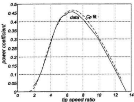
Figure 3.7 Power coefficient curve,  $C_p(\lambda)$ .
