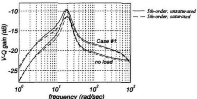
Figure 4.25 SG + exciter Bode plot, reactive power to voltage gain.
