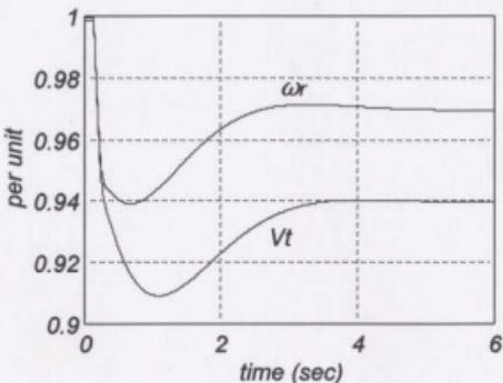
Figure 4.20 SG + exciter open circuit voltage, constant  $V_R$ .
