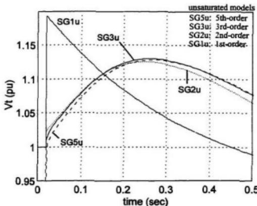
**Figure 4.5 SG voltage response to WT disconnect, Case #1.**
