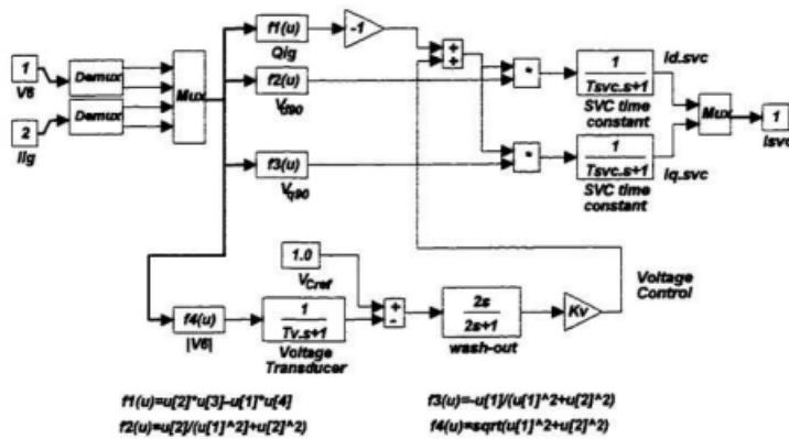
Figure A.17 Static VAR compensator model.
