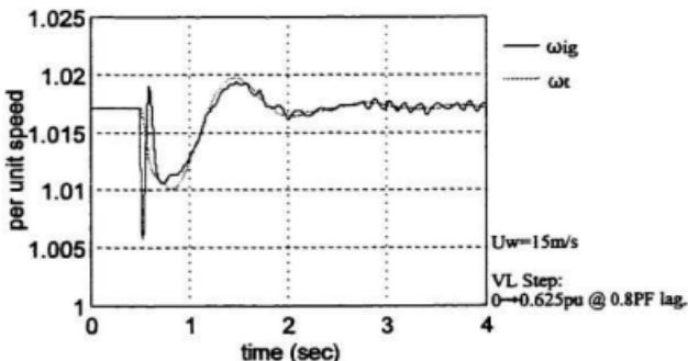
Figure 5.12 *Wind-only* WT swing with phase detector.
