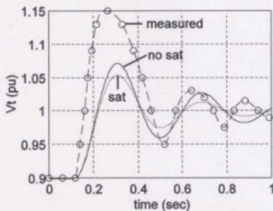
Figure 4.17  $V_{ref}$  step,  $K_F = 0.005$ .
