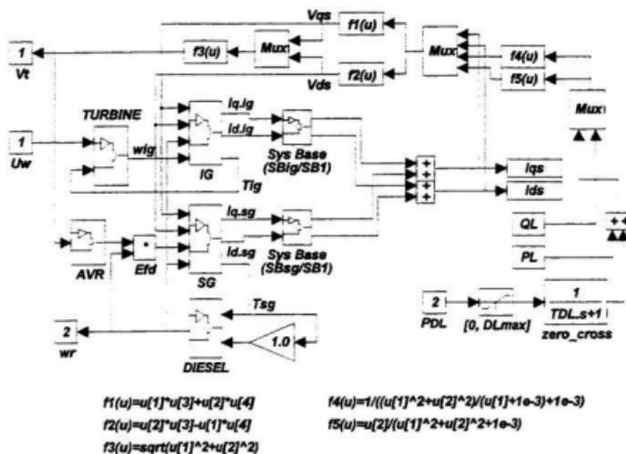
Figure A.8 Full-order wind-diesel subsystem model.
