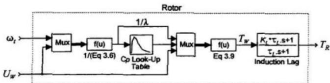
**Figure 3.9 Complete aerodynamic model of the wind turbine.**
