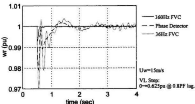
Figure 5.9 *Wind-only* frequency response to a (diesel) full load step.
