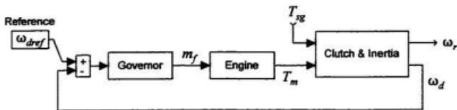
**Figure 3.2 General mechanical model of the diesel generator.**
