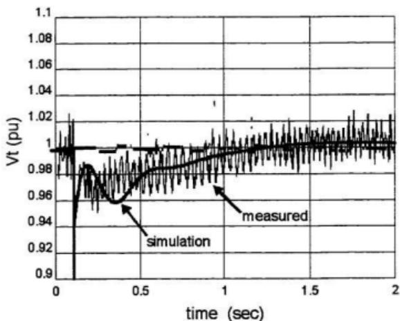
Figure 4.29 Voltage, Diesel A, load  $0.05 \rightarrow 0.64\text{pu}$ ,  $\tau'_{q0} = 35\text{ms}$ .
