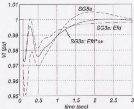
Figure 4.23 SG response to speed proportional field.
