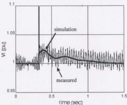
Figure 4.18 Voltage, Diesel A, load:  $0.35 \rightarrow 0.03$  pu ( $K_F=0.02$ ).
