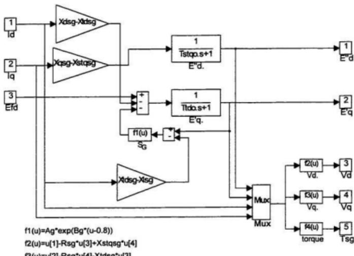
Figure A.5 SG2: 2nd-order synchronous generator model.
