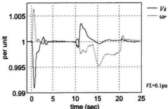
Figure 5.20 Flicker with added capacitor bank.
