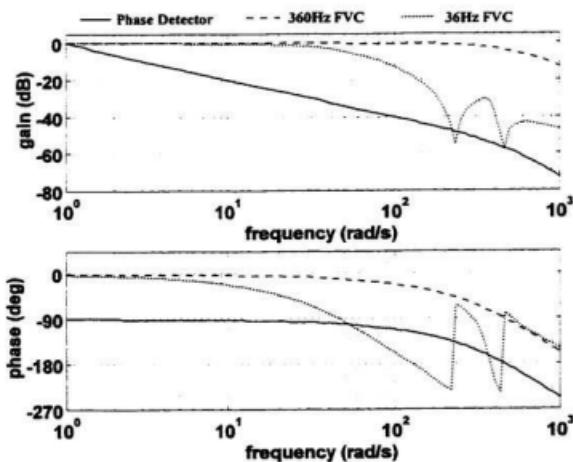
Figure C.5 Frequency response of the frequency detectors.
