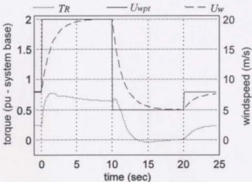
Figure 5.16 Windspeed used for voltage flicker test.
