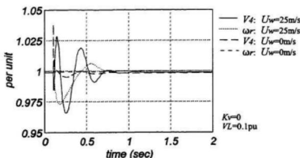
Figure 5.22 Wind turbine disconnect with SVC ( $K_v=0$ ).
