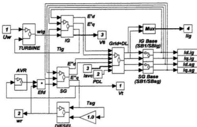
Figure A.15 Reduced-order wind-diesel subsystem with SVC connection.
