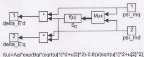
Figure A.7(b) Saturation subsystem of IG2 model.
