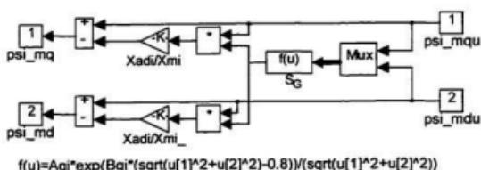
Figure A.10(b) Saturation subsystem of IG4 model.
