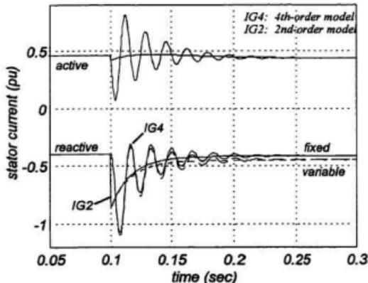
Figure 4.33 IG current response to a +5% voltage step.
