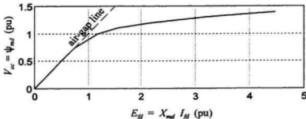
Figure 3.11 Generator open circuit voltage vs. field current.
