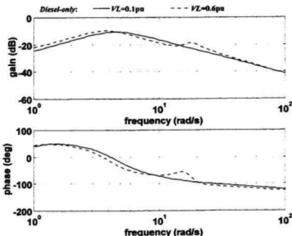
Figure C.4 Bode diagram of *diesel-only* configuration.
