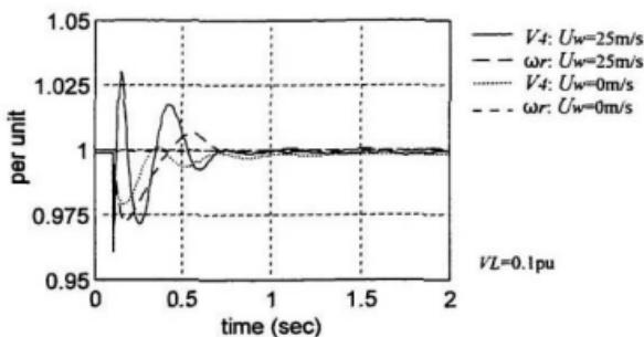
Figure 5.18 Wind turbine disconnect with capacitor bank.
