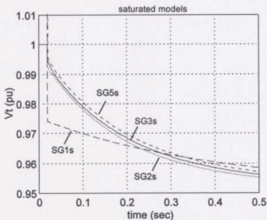
Figure 4.10 SG voltage response to WT disconnect, Case #3.
