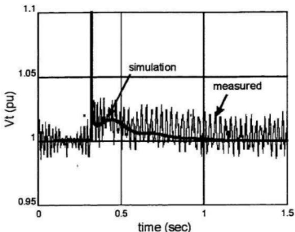
Figure 4.28 Voltage, Diesel A, load:  $0.35 \rightarrow 0.03\text{pu}$ ,  $\tau'_{q0} = 35\text{ms}$ .
