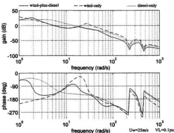
Figure 5.8 Bode diagram of 36Hz FVC dump load control loop.
