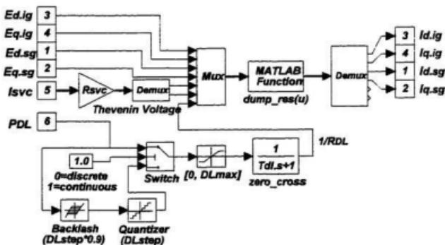
Figure A.16 Network admittance model with SVC connection.
