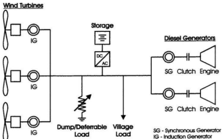
Figure 1.1 General wind-diesel system.
