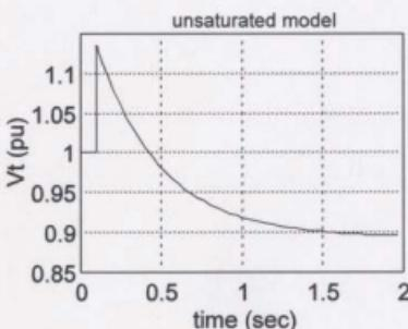
Figure 4.13 1st-order SG, load:  $(.4+j.3) \rightarrow (.96)$  pu.
