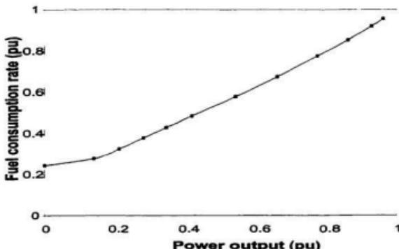
Figure 1.2 Typical diesel generator fuel consumption.
