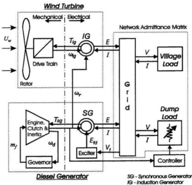
Figure 3.1 Block diagram of the HPNSWD model.
