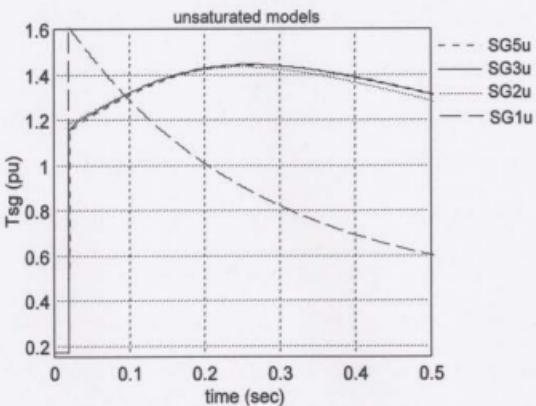
Figure 4.7 SG torque for WT disconnect, Case #1.
