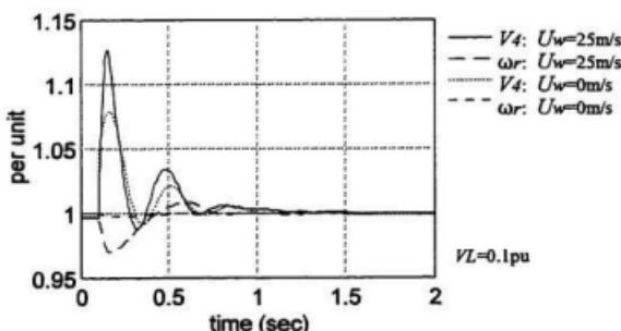
Figure 5.15 Wind turbine disconnect with synch. generator only.
