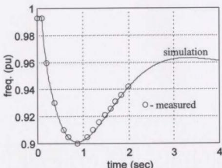
Figure 4.1 Speed of Diesel A for a +0.64 pu load step.
