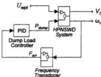
Figure 5.5 Dump load controller block diagram.
