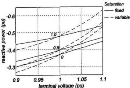
Figure 4.32 V-Q curves for 0, 0.5 & 1 pu active power.
