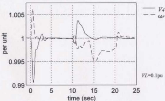
Figure 5.17 Flicker with synchronous generator only.
