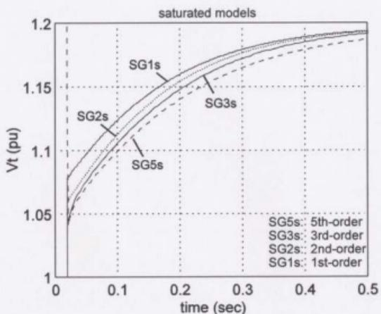
Figure 4.9 SG voltage response to WT disconnect, Case #2.
