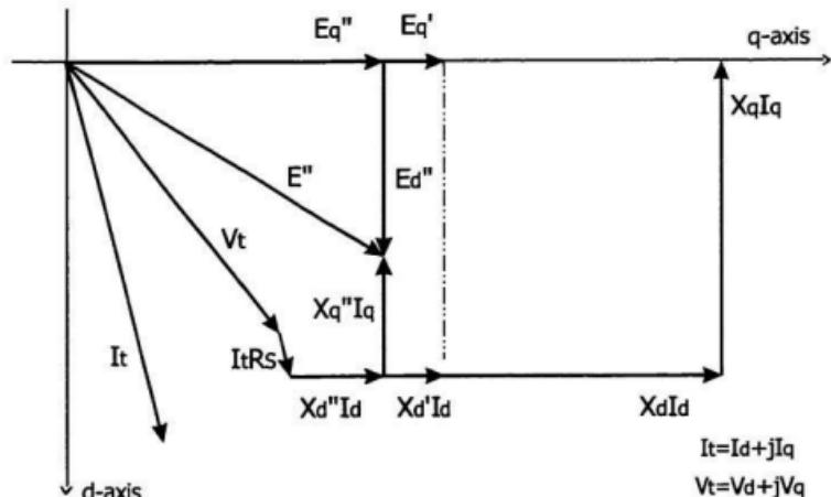
Figure 3.13 Synchronous generator phasor diagram.
