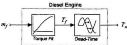
Figure 3.3 Diesel engine dynamic model.
