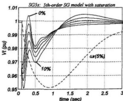
Figure 4.26 Voltage response: increasing  $\omega_r$  transients.
