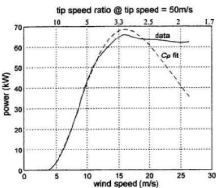
Figure 3.8 Wind turbine power curve.
