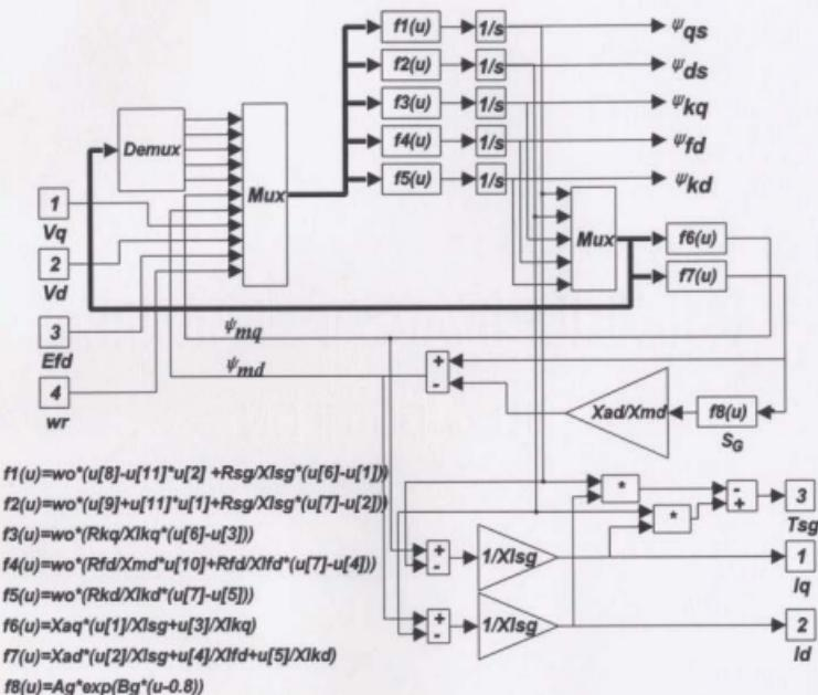
Figure A.9 SG5: full-order synchronous generator model.
