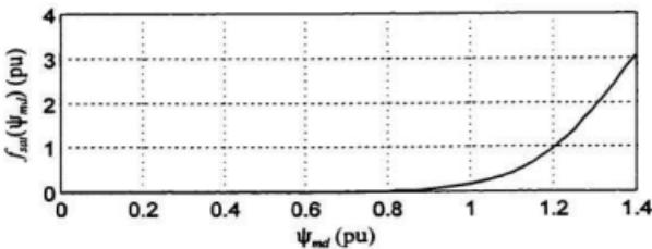
Figure 3.12 Generator saturation function.
