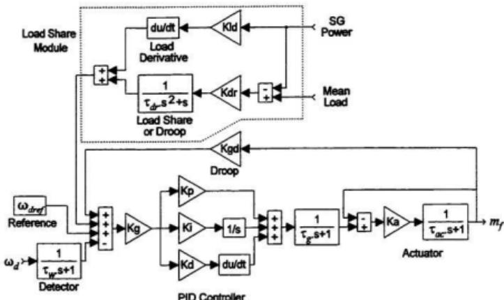
Figure 3.5 Functional diagram of the Barber-Colman governor system.
