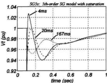
**Figure 4.27 Voltage, Diesel A +0.64pu load step.**
