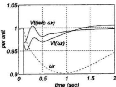
Figure 4.22 SG voltage, w/ & w/o speed terms.
