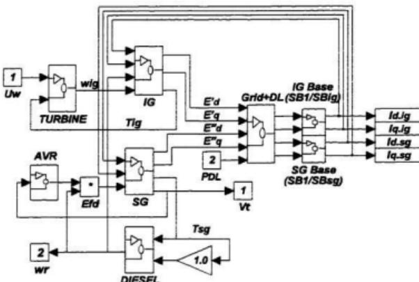
Figure A.2 Reduced-order wind-diesel subsystem model.
