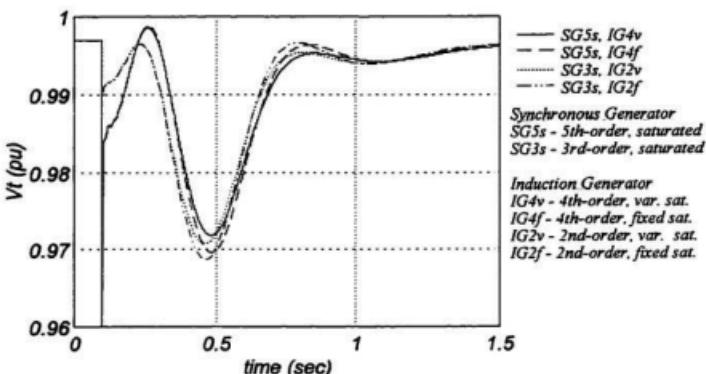
Figure 4.35 HPNSWD voltage response, +0.4 pu load step.
