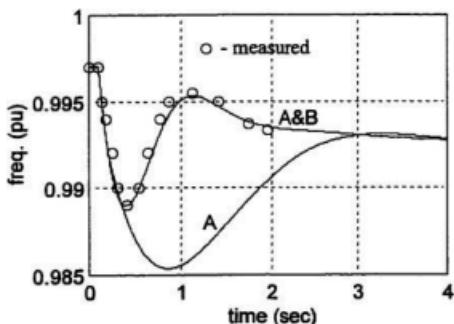
Figure 4.3 Diesels A&B speed for a +0.08 pu load step.
