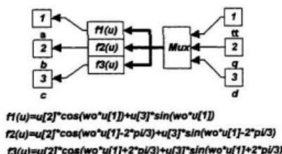
Figure D.4 Inverse Park transformation subsystem.
