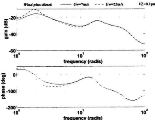
Figure C.2 Bode diagram of *wind-plus-diesel* configuration.
