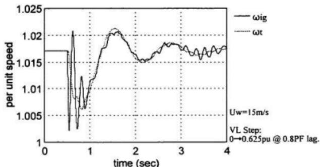
**Figure 5.13** *Wind-only WT swing with 36Hz FVC.*
