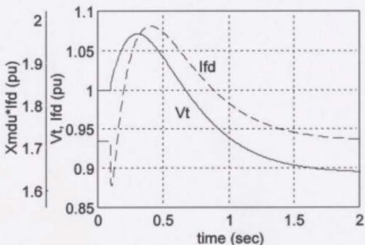
Figure 4.12 SG 3rd-order unsaturated, load:  $(.4+j.3) \rightarrow (.96)$  pu.
