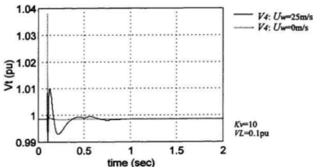
Figure 5.24 Wind turbine disconnect with SVC ( $K_v=10$ ).
