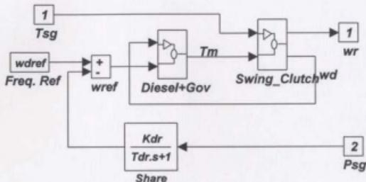
Figure A.11(a) Diesel generator mechanical model.
