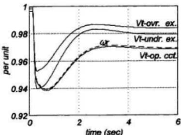
Figure 4.21 SG response to rotor speed variation.
