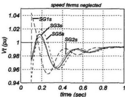
Figure 4.30 SG + exciter,  $\tau'_{q0} = 35\text{ms}$ , +0.64pu load.
