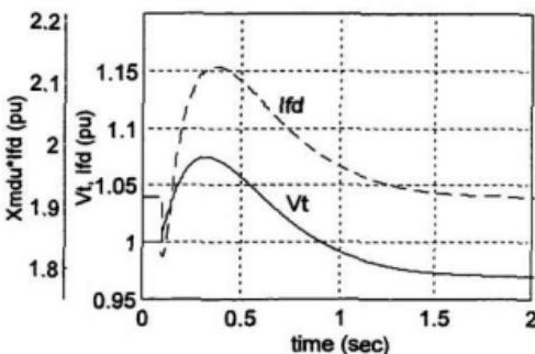
Figure 4.14 SG 3rd-order, saturated, load:  $(.4+j.3) \rightarrow (.96)$  pu.
