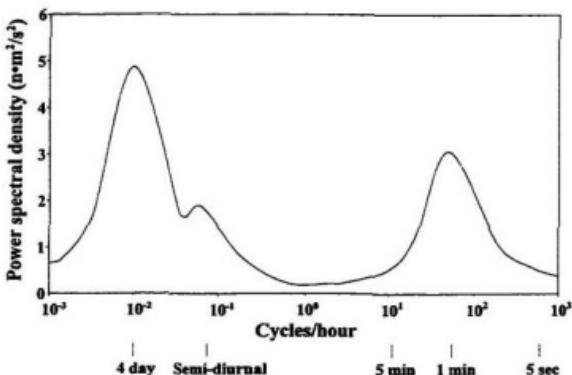
Figure 1.3 Spectrum of horizontal windspeed at Brookhaven, NY.
