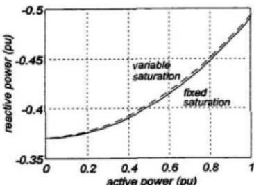
Figure 4.31 IG steady-state P-Q curve.
