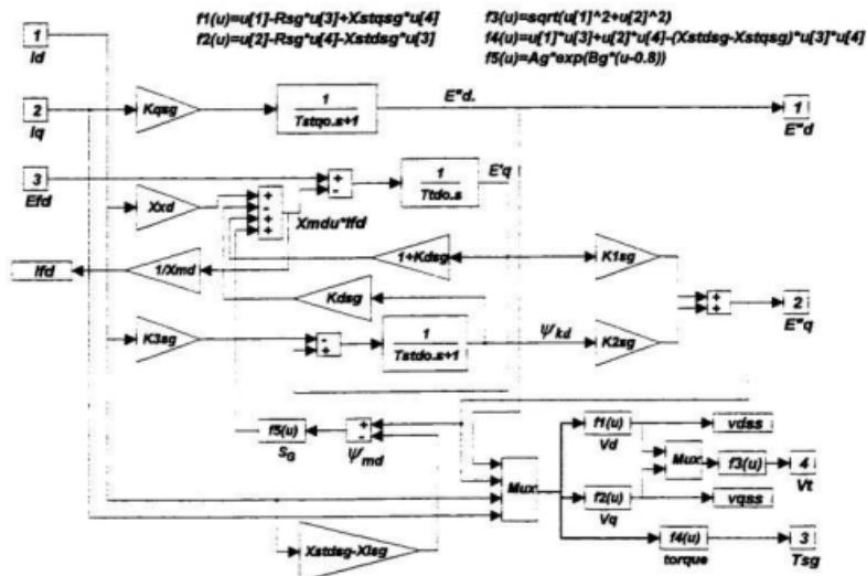
Figure A.4 SG3: 3rd-order synchronous generator model.
