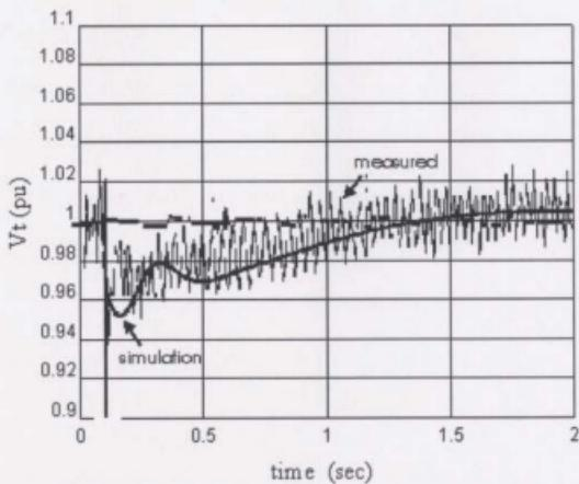
Figure 4.19 Voltage, Diesel A, load:  $0.05 \rightarrow 0.64$  pu.
