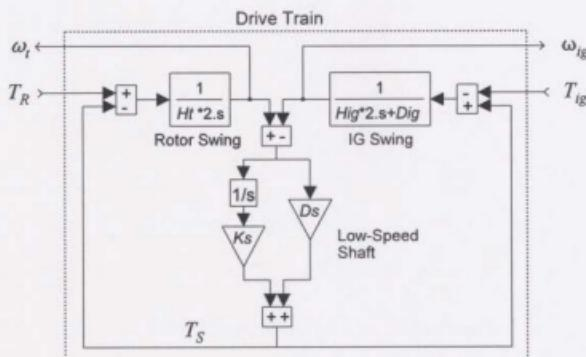
Figure 3.10 Wind turbine drive train model.
