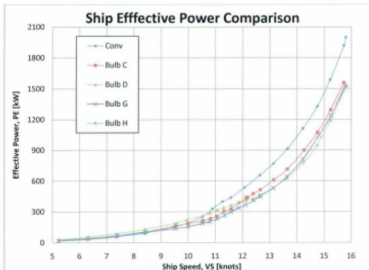
Figure 32: Ship Effective Power Vs. Speed
