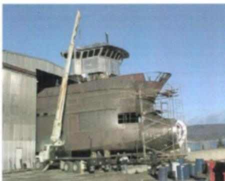
**Figure 2: Fabrication of Concept Bulbous bow**
