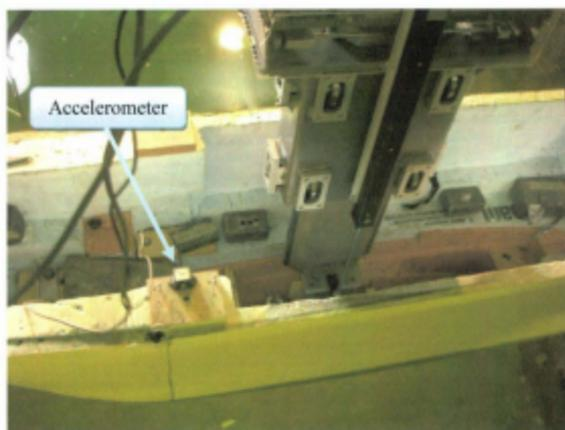
**Figure 21: Location of Accelerometer**
