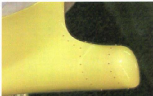
**Figure 19: Example of Turbulence Studs**
