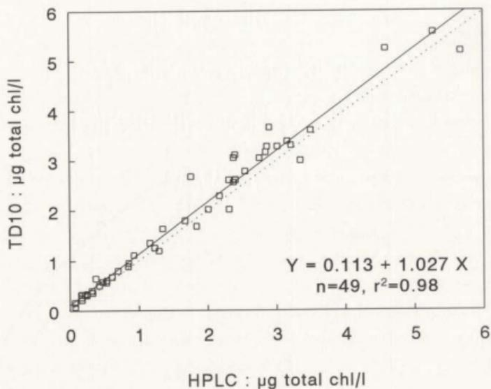
Figure 4.17. Relationship between standard fluorometric (TD10) and HPLC measurements of total chloropigments ( $\mu\text{g/l}$ ) in seston <505 $\mu\text{m}$  collected during the spring 1988. Dotted line represents a 1:1 ratio.
