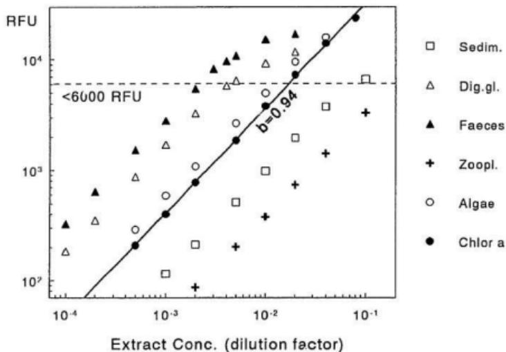
Figure 2. 1. Turner Designs Model 10 fluorescence detector response for diluted extracts of marine sediment, mussel digestive gland, mussel faeces, zooplankton, lab algae (*Chaetoceros* sp.) and chlorophyll *a* standard.
