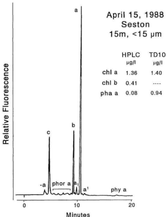
Figure 4.16. HPLC fluorescence profile of pigments extracted from seston <15 $\mu$ m collected from a depth of 15 m on April 15, 1988. Peak identities are: -a (chlorophyllide a), c (chlorophyll c), b (chlorophyll b), a (chlorophyll a), a<sub>1</sub> (allomers of a), a' (epimers of a), phor a (phaeophorbide a-types), phy a (phaeophytin a). Note the TD10 overestimation of phaeopigments (pha) in the presence of high levels of chlorophyll b.
