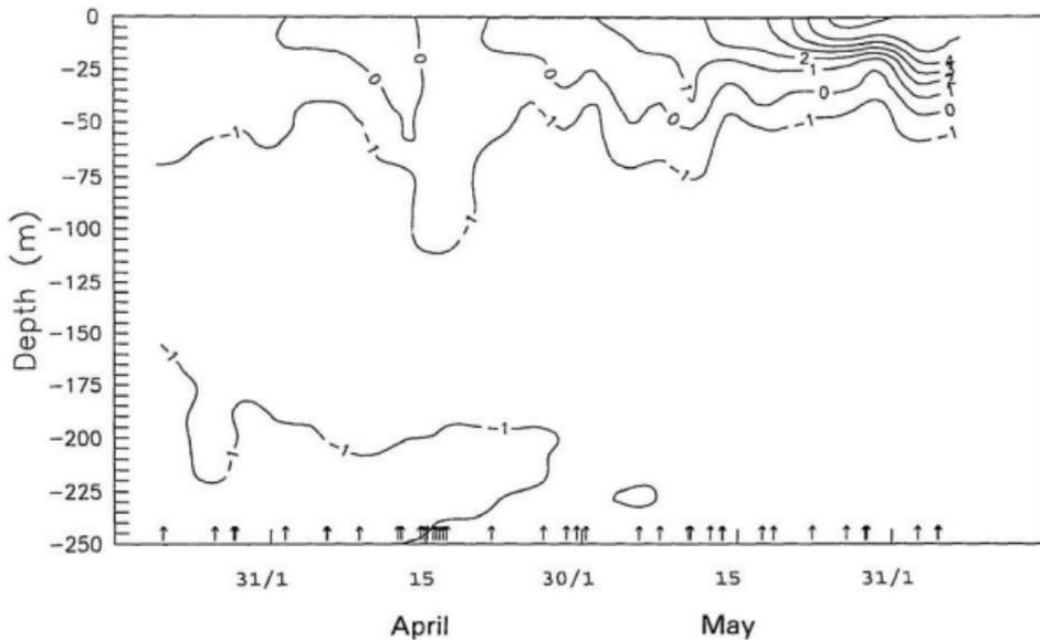
Figure 4.3. Time-depth plot of temperature ( $^{\circ}\text{C}$ ) at the Conception Bay sampling site during mid-March to early June, 1988. Measurements were determined using a Seabird SBE 20 CTD. Arrows indicate dates of CTD casts.
