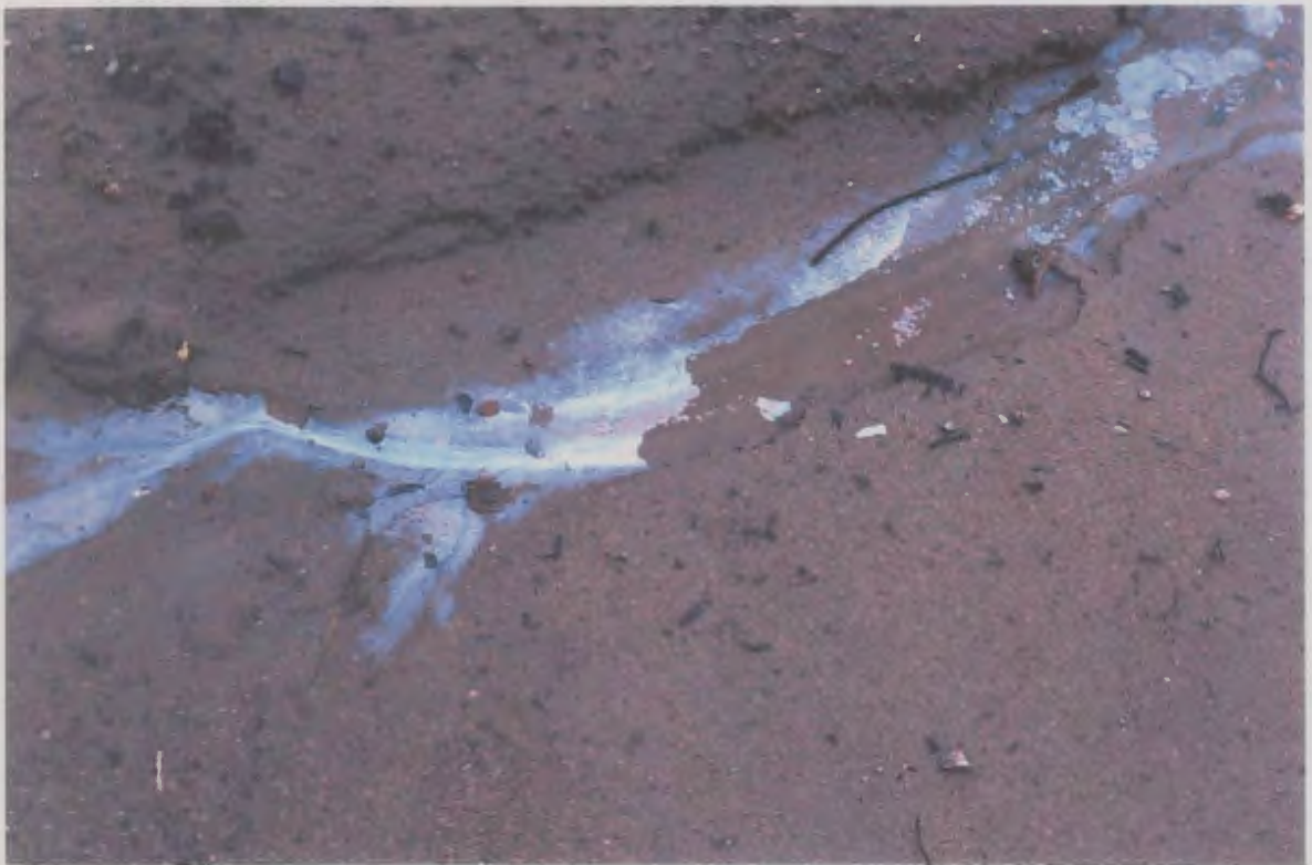
Figure 2.6: Manganese (Mn) slick at SW1. Note the sharp, jagged edges; evidence that once disturbed, the slick will not congeal again, unlike the petroleum hydrocarbon slick in Figure 2.5.
