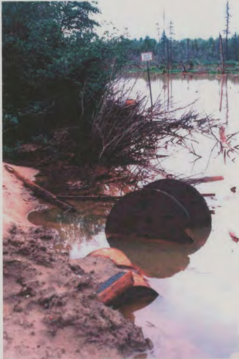
Figure 2.10: SW4 sampling site showing discarded and rusting 45-gallon drum and electrical cable reel. Note the opaqueness and orange water colour.
