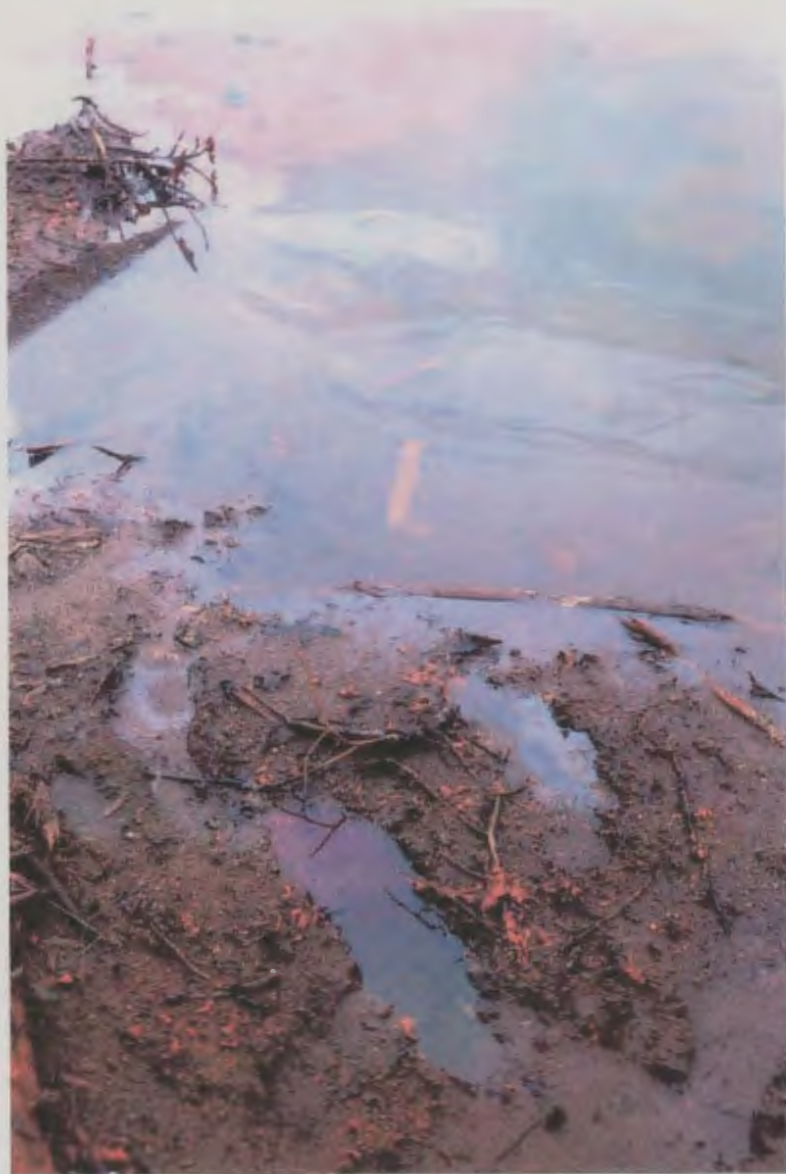
Figure 2.5: Petroleum hydrocarbon sheen at SW1. Note the orange iron precipitate.
