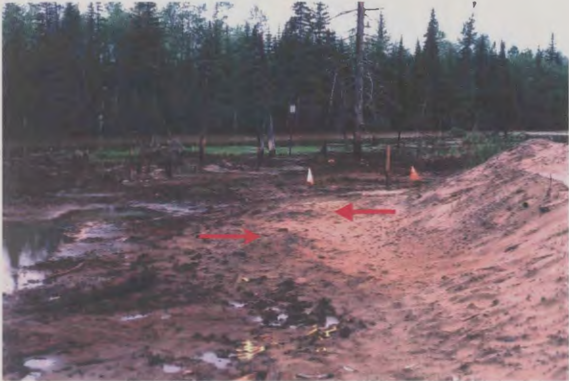
Figure 2.11: SW4 shoreline. Note the high water contamination marks (red arrows) on the sand. Orange flags indicate sediment sampling sites from previous consultants.
