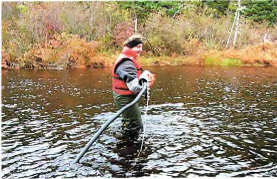
Figure 2.7 WRMD Personnel Installing a Hydrolab Datasonde in Peter's River
