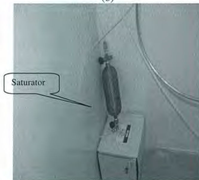
Figure (7.4) Components of the gas hydrate apparatus: a) b) parts located in the small chamber (coil, separator, saturator); c) Parts located in the large chamber (orifice, pipe)
