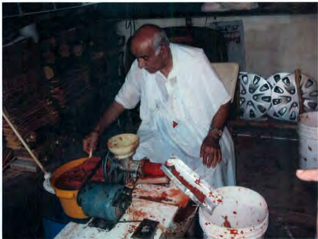
Figure 23: My nonno and his homemade Juice Extractor/Sausage Maker. The bucket on the right is collecting the skin and core of the tomatoes. A bucket facing him (not visible in photo) is collecting the juice. (Photo by L.S.)
