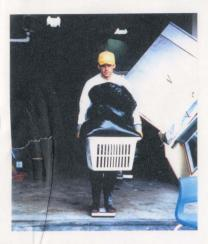
Photo 5: Determining the overall weight of a quartered sample.
