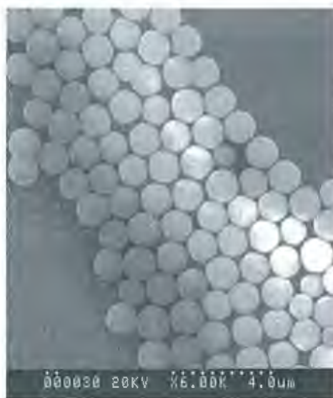
(b) SEM image of NL6. 1.27 \mu\text{m} diameter (4.1% polydispersity).
