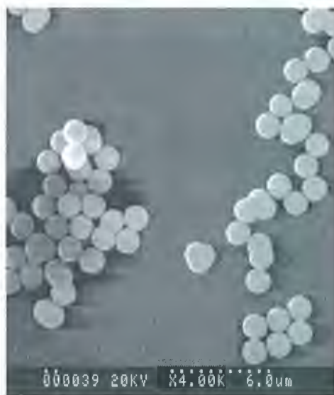
(a) SEM image of NL4. Lots of non-spherical aggregates.
