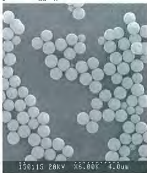
(c) SEM image of NL8. 1.14 \mu\text{m} diameter (3.4% polydispersity).
