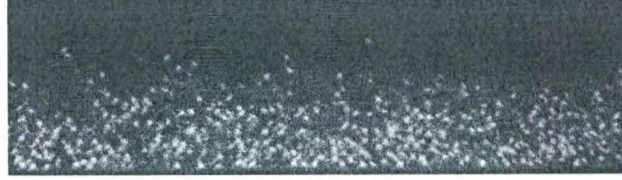
Figure 1.7: x - z view confocal image of core-shell silica colloids. Rebuilt confocal image for the side view of sedimented 0.77 \mu\text{m} silica colloids, where zoomed ratio is x:z = 2:1 .
