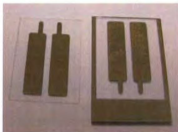
Figure 2.22: The gold-film-electrodes coated on glass slides for two-electrode linear field cell.
