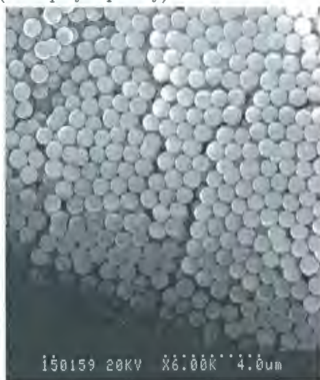
(d) SEM image of NL9. 0.77 \mu\text{m} diameter (3.8% polydispersity).
