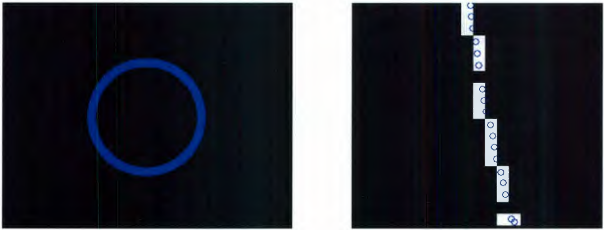
Figure 6.12: Edge points of the sphere refined through subpixel interpolation (a) Location of edges with subpixel accuracy (b) Closer view of the location of edges represented by blue circular points
