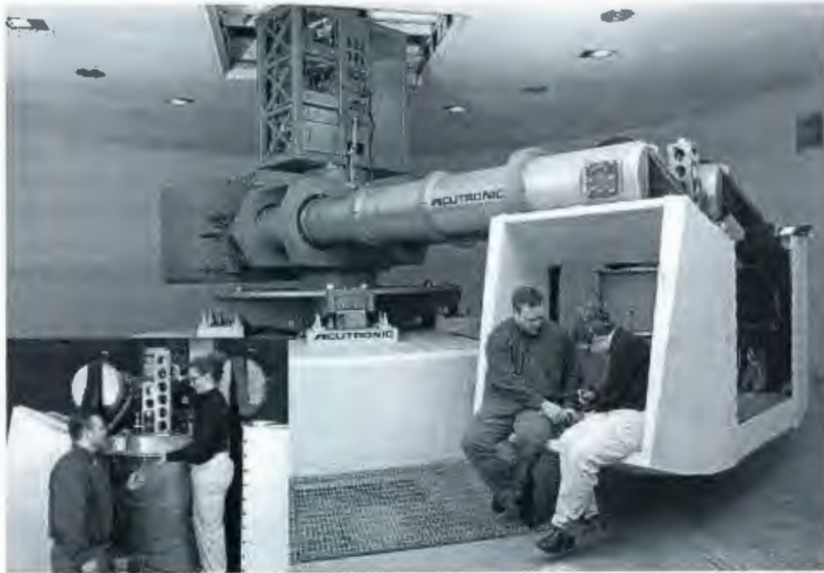
Figure 4.1: C-CORE Acutronic 680-2 Geotechnical Centrifuge.
