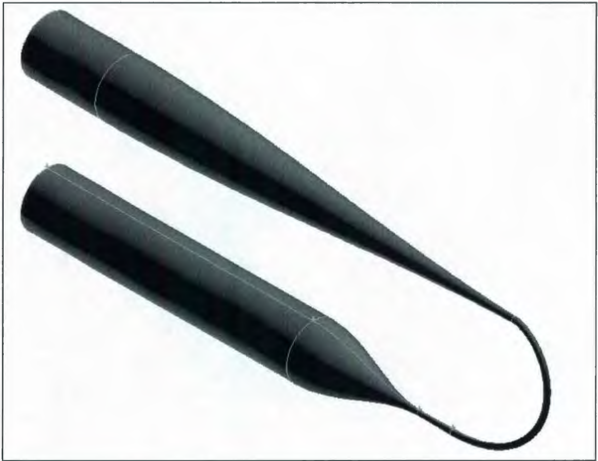
Figure 4.3 A Typical three dimensional geometry: nozzle with extended U-shaped section.
