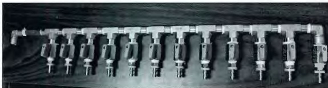
Figure 6.7 Pressure measurement manifold. The elbow on the far left is to be connected to the pressure gauge.
