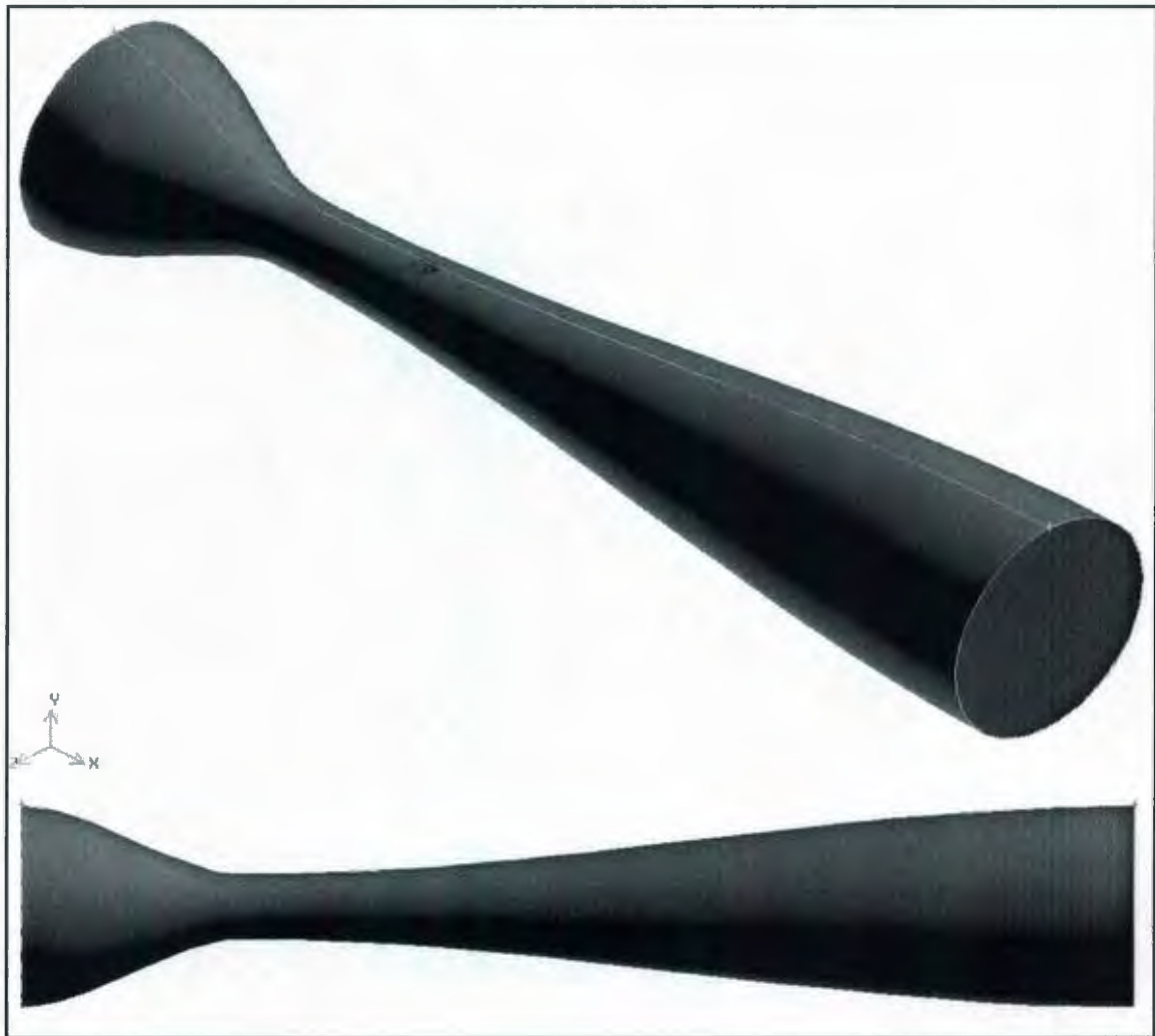
Figure 4.1 Two dimensional geometry, used as an axis-symmetric body to simulate a typical nozzle
