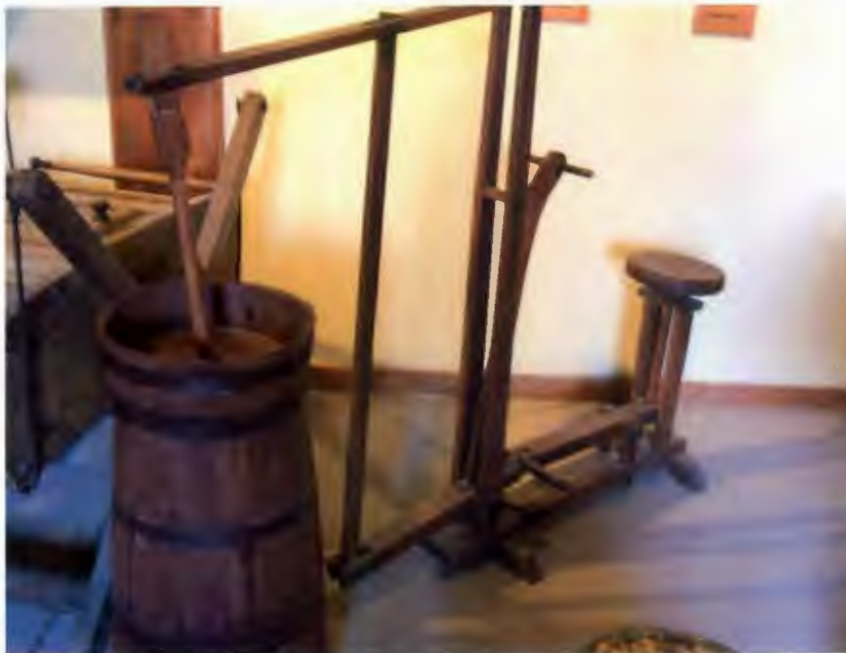
Fig. 49) Wooden, ride-on dasher churn attachment, circa 1880s. MCFP 976.15.01
