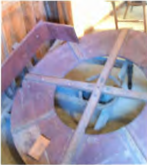
Fig. 52) Horizontal wooden power-wheel, from St. Mary's, Ontario. MCFP unnumbered.
