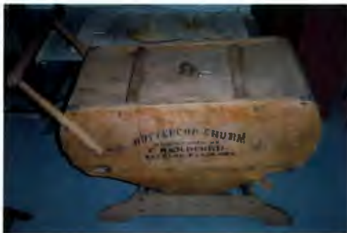
Fig. 25) Early Ontario upright dasher churn shown as one piece. NMSTC 660338.1-4.
