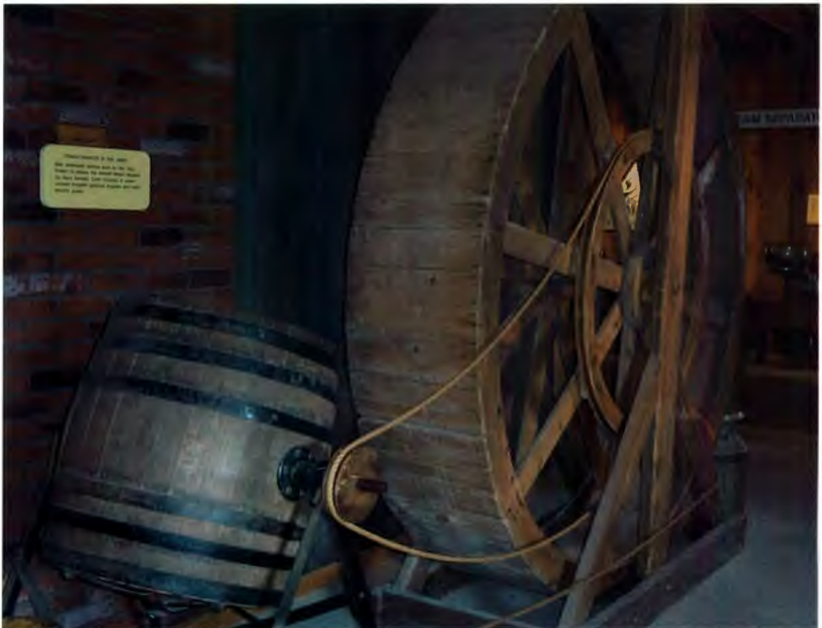
Fig. 53) Eight-foot high, vertical, wooden power-wheel attached to end-over-end barrel churn, from Staffa, Ontario. MCFP unnumbered.
