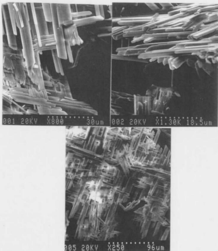
Figure 3.1 a, b, and c: Scanning electron micrographs of solid reaction products obtained from iron phosphate and aqueous sodium phosphate ( $\text{Na/P}=2.15$ ) at  $250^{\circ}\text{C}$  for three weeks.
