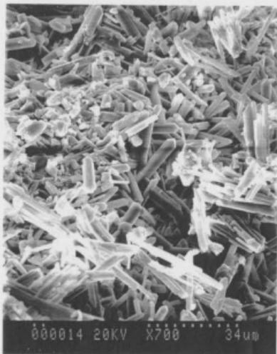
Figure 3.4 a and b : Scanning electron micrographs of solid reaction products obtained from magnetite and aqueous sodium phosphate ( $\text{Na/P}=2.15$ ) at  $250^{\circ}\text{C}$  for three weeks.
