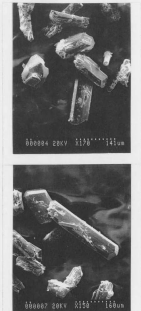
Figure 3.11 a and b: Scanning electron micrographs of solid reaction products obtained from flow experiment involving a stainless steel vessel and aqueous sodium phosphate at 288°C for 17 days.
