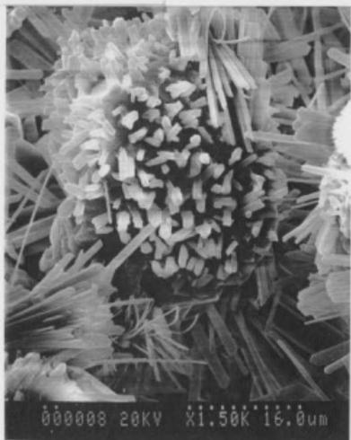
Figure 3.3 a, b, and c: Scanning electron micrographs of solid reaction products obtained from hematite and aqueous sodium phosphate ( $\text{Na/P}=2.5$ ) at  $250^{\circ}\text{C}$  for three weeks.
