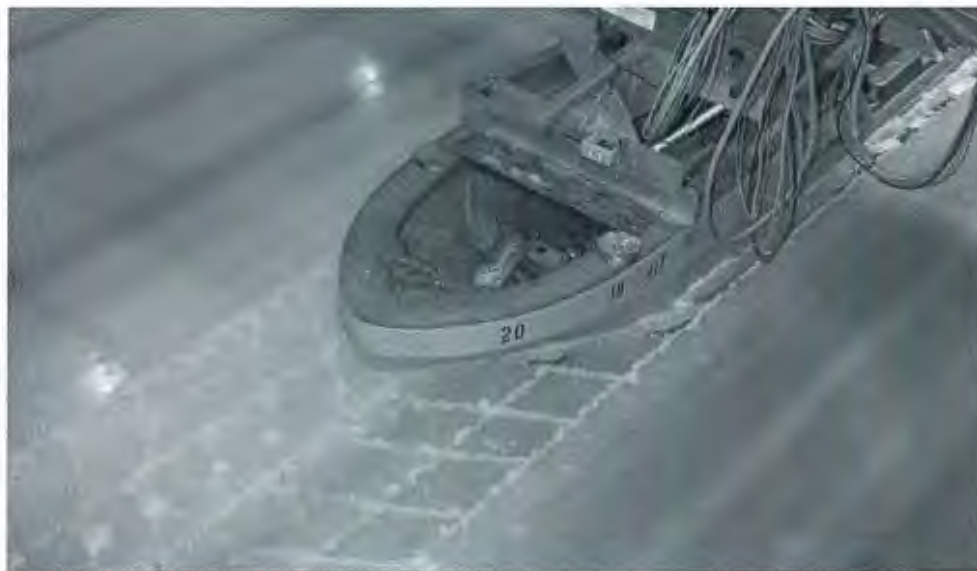
Figure 6.5 PMM Terry Fox model test run in pre-sawn ice (Derradji et al., 2004a)
