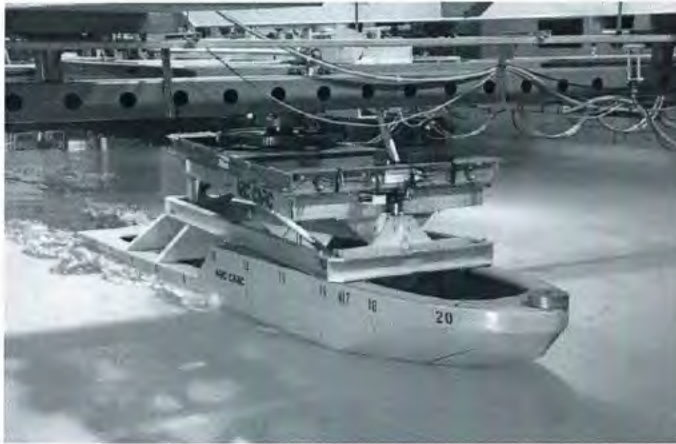
Figure 6.4 PMM Terry Fox model test run in level ice (Derradji et al., 2004a)
