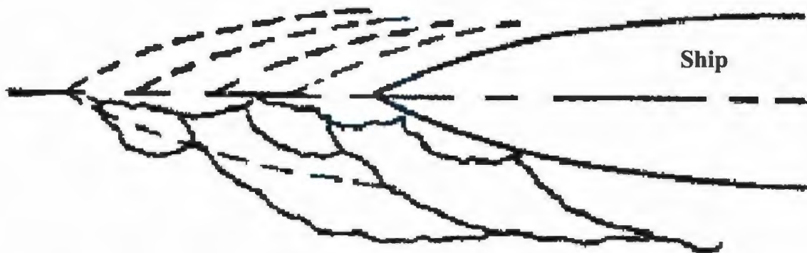
Figure 3.10 Sketch of icebreaking process by the bow of an icebreaker
