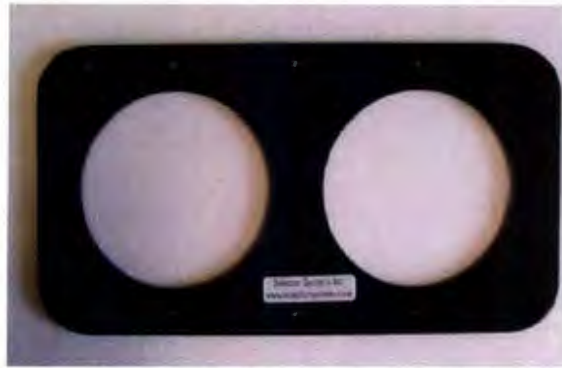
Figure 7.1 The circular escape mechanism tested and in voluntary use in the Newfoundland and Labrador snow crab ( Chionoecetes opilio ) fishery. The mechanism measures 250 x 140 millimetres (length and width) with two identical escape opening having an inside diameter of 95 mm each. (Source: Keats et al. , 2008).
