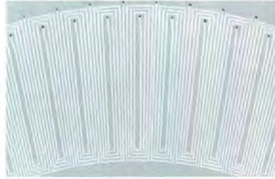
Figure 4.11: The designed PCB stator winding
