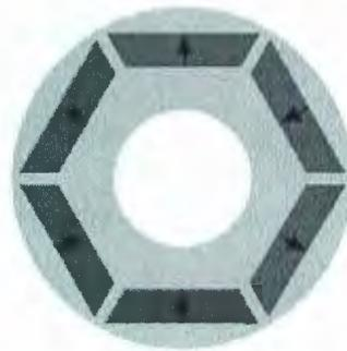
Figure 1.5: Interior magnet rotor
