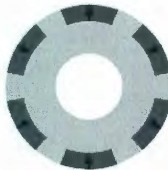
Figure 1.7: Inset magnet rotor
