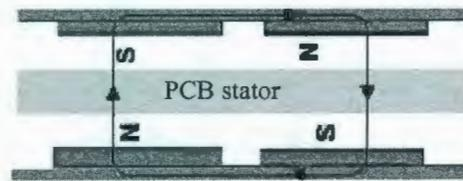
Figure 4.2: 2D view of the double sided AFPMG with PCB stator
