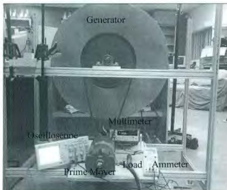
Figure 3.11: Test setup for first prototype
