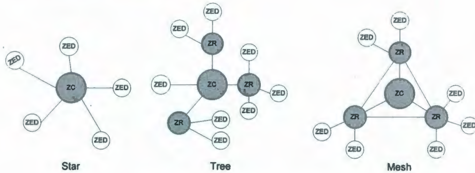
Fig. 2.6 Network topology of Zigbee.
