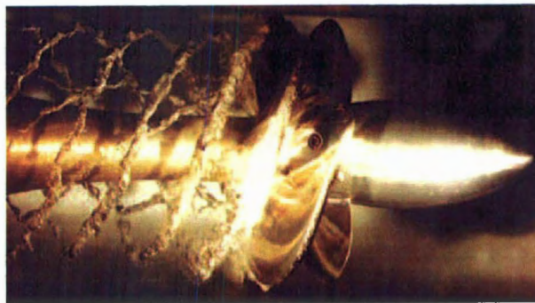
Figure 1-1: Cavitation flow of a propeller (DGA-DCE)
