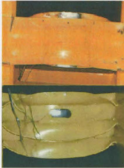
Figure 3.7: View of deformed test specimen showing plate bending between stiffeners (top) and buckled stiffeners (bottom)
