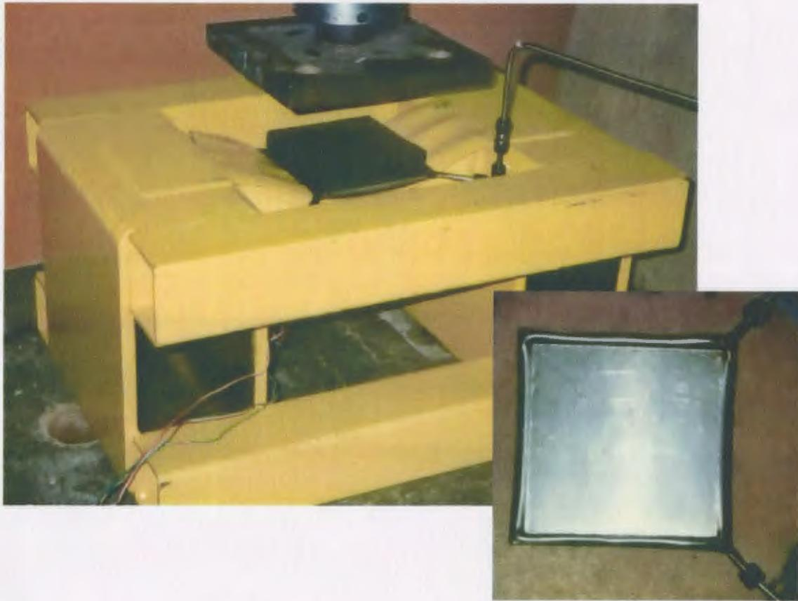
Figure 3.6: Loading ram/flatjack interaction and resulting flatjack indentations (inset)
