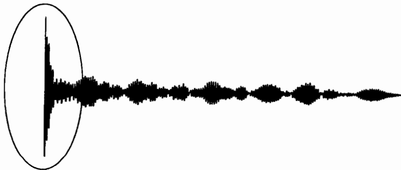
Figure 4.14.c. The auto-correlation function (half side, only circled part is used in the analysis).
