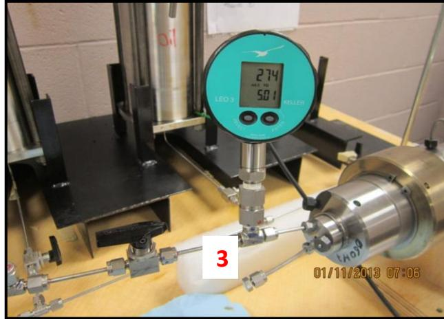
Figure 3.14 Keller LEO3 pressure transducer
