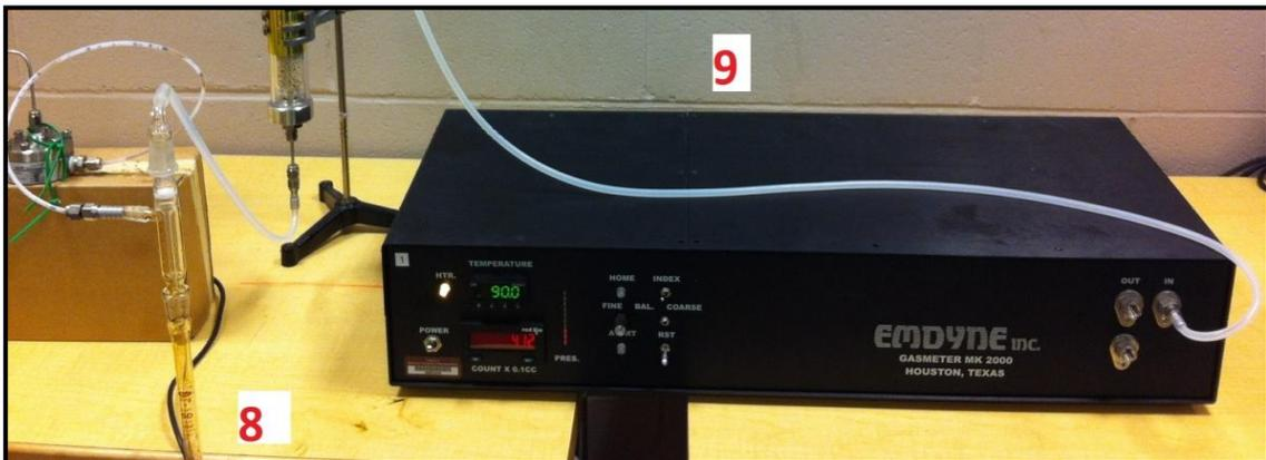
Figure 3.13 Coreflooding outlet section (8: phase separator, 9: Emdyne MK 2000 gasmeter)
