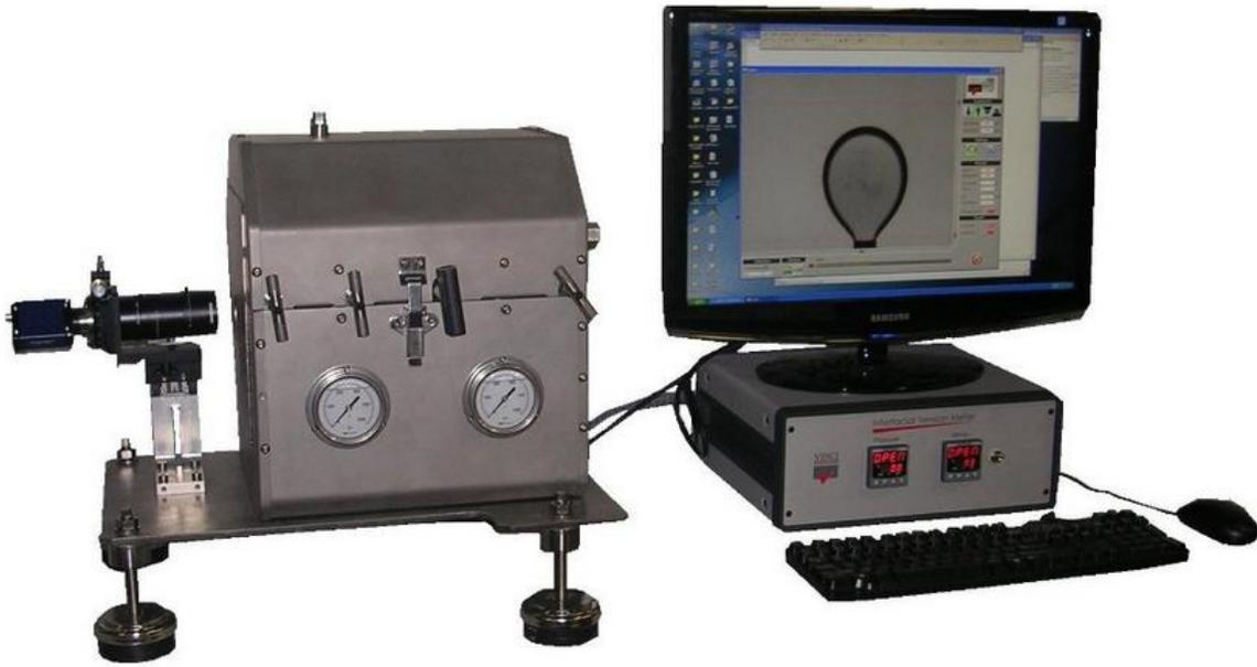
Figure 3.6 Vinci Interfacial Tension (IFT 700) apparatus
