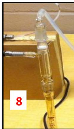
Figure 3.16 Custom made three phase separator
