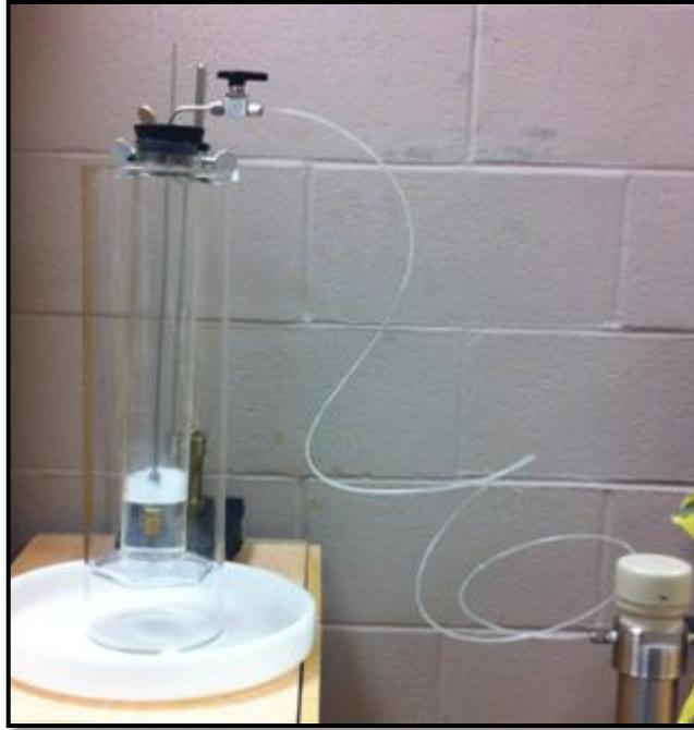
Figure 3.2 Air injection apparatus in the glass bath cylinder
