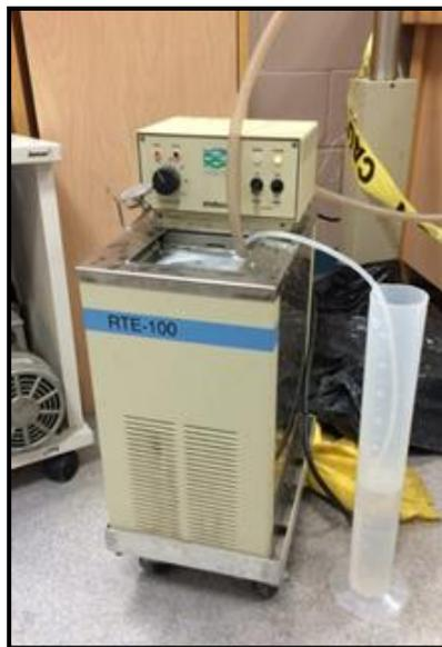
Figure 3.3 Neslab RTE-100 water bath
