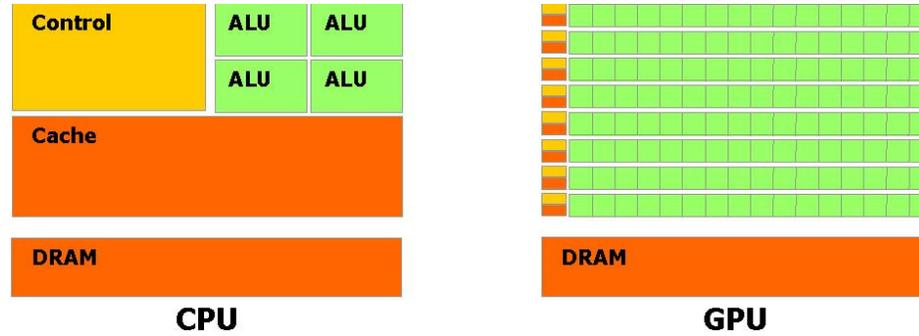
Figure 2.8: Different structures of GPU and CPU [24]
