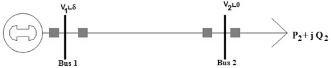
Figure 3.1 Model of a simple transmission system
