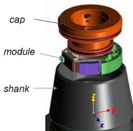
Figure 8 Assembly Drawing Showing the Approximate Arrangement of the Module Prior to Implantation in the End of a Bit Shank [16]
