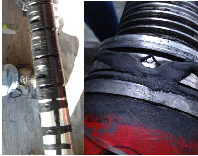
Figure 60 Wrapped measurement tool (Left) and damaged seal rings (Right)
