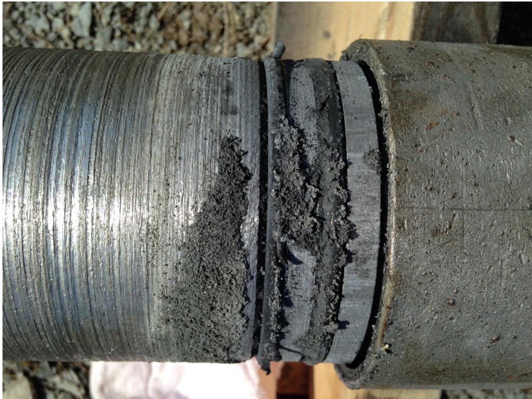
Figure 59 Seal was damaged after test
