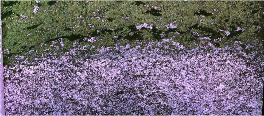
Figure 6-6: Layered sample, predominantly pyroxene (top) and feldspar (below) in sample CBD-11-07-12. Pyroxene exhibits many fractures perpendicular to mineralogical layering, whereas feldspars do not appear to contain any fractures. Width= 25 mm.
