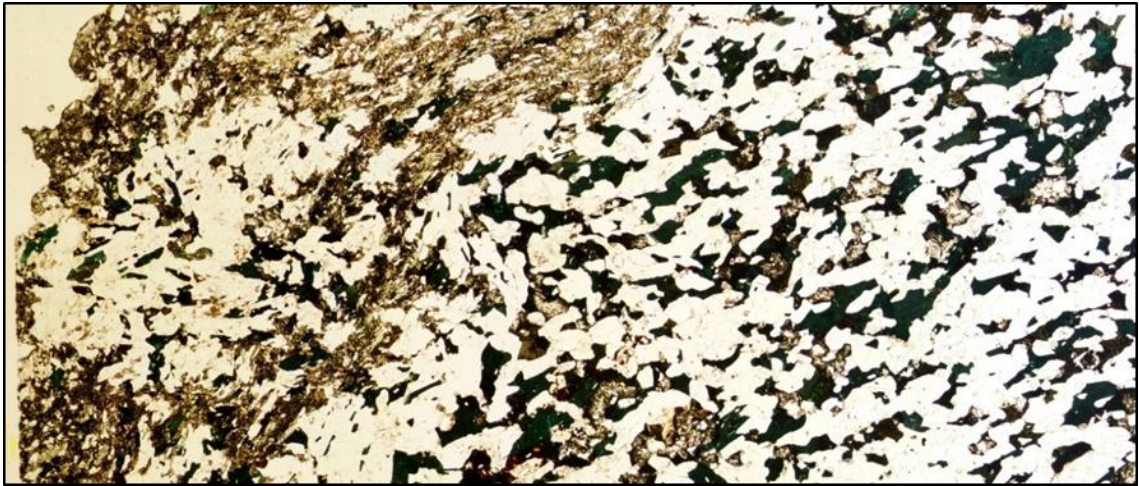
Figure 2-10: Contact area between two subunits of leucosyenite, pyroxene-rich (2a-left) versus amphibole-rich (2b-right). Field of view is ~24 mm. From sample CBD-10-01-24.
