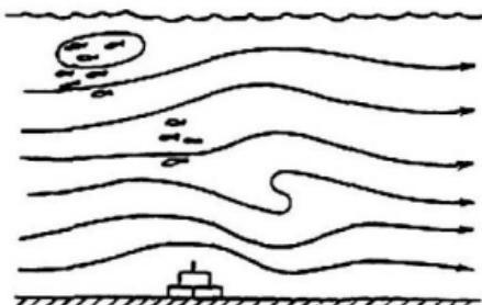
Figure 2.5. Lee Wave due to Artificial Reefs (Nakamura, 1985)
