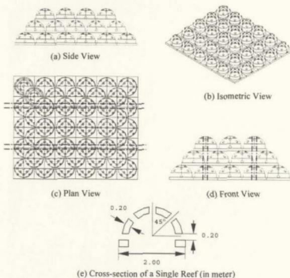
Figure 5.1 Typical Three Dimensional Reef Arrangement
