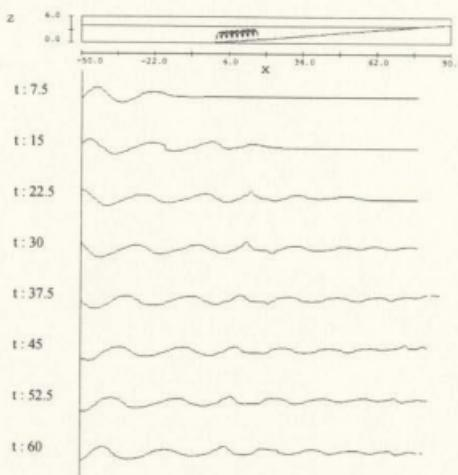
Figure 5.9 Wave Profile with Twenty-four Reefs, T: 4.0 sec
