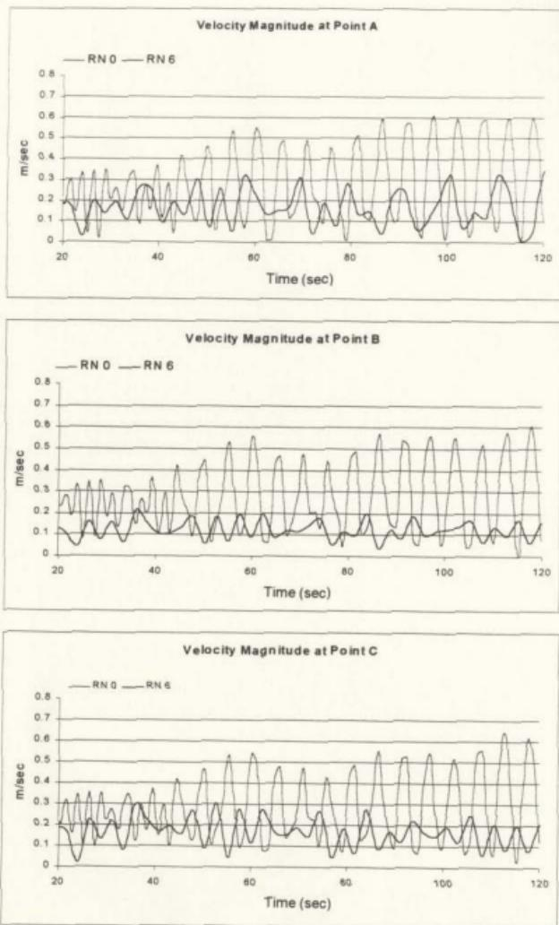
Figure 4.26. Velocity Magnitudes Time Series for Six Reefs at Points A, B, and C
