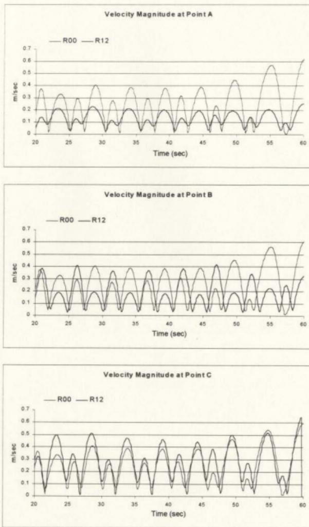
Figure 5.22 Velocity Magnitude Time Series for Twelve Reefs at Points A, B, and C
