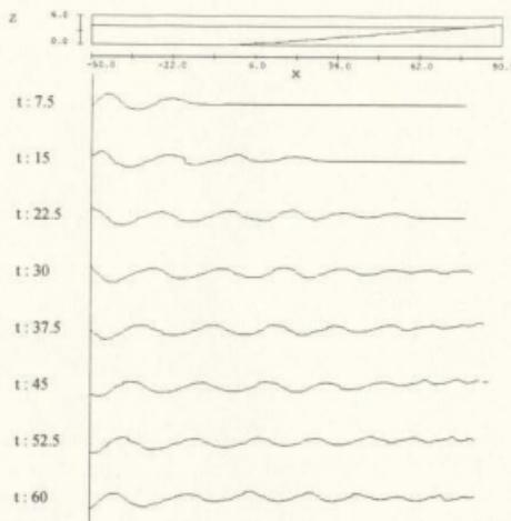
Figure 5.8 Wave Profile without Reefs, T: 4.0 sec
