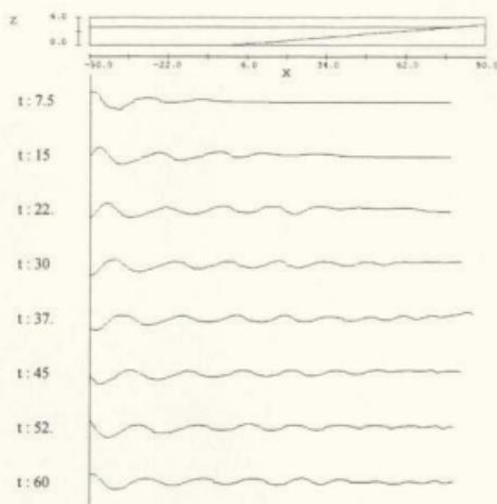
Figure 5.10. Wave Profile without Reefs, T; 3.5 sec
