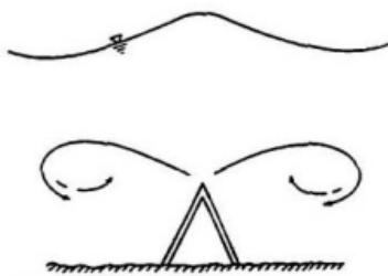
Figure 2.6. Turbulent Wake due to Wave Action (Takeuchi, 1991)
