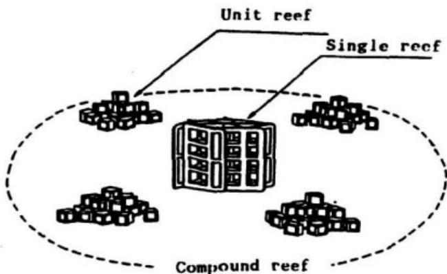
Figure 2.11. Typical Size Scales of Artificial Reefs (Kakimoto, 1991)
