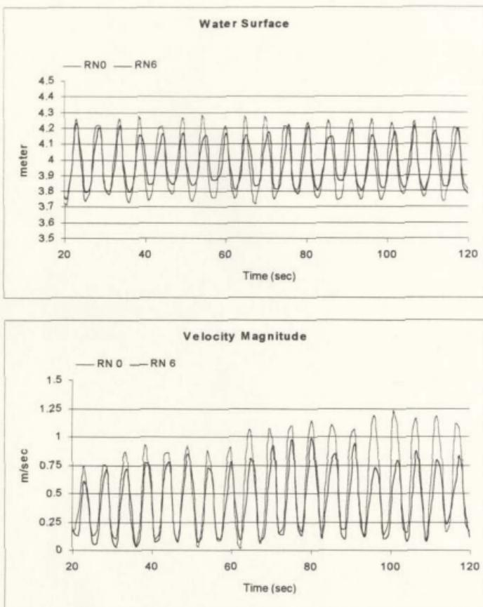
Figure 4.15 Water Surface Profile and Surface Velocity Magnitude Time Series for Six Reefs at  $x:+15.0\text{m}$
