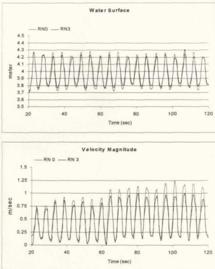
Figure 4.14 Water Surface Profile and Surface Velocity Magnitude Time Series for Three Reefs at  $x:+15.0\text{m}$
