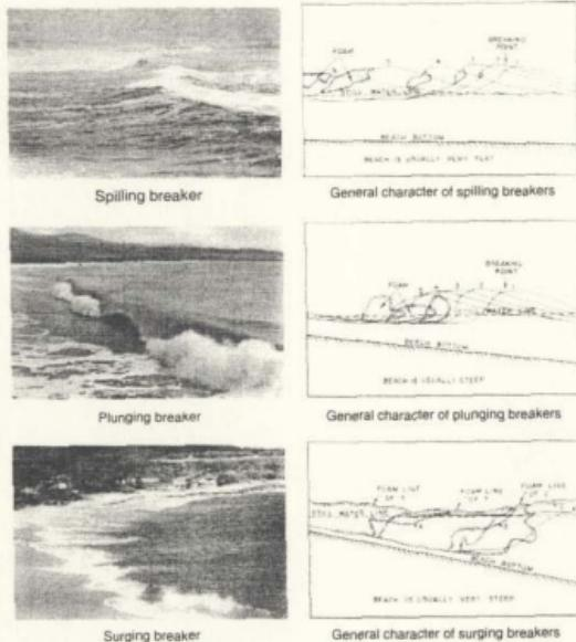
Figure 4.5 Types of breaking waves on the shore
