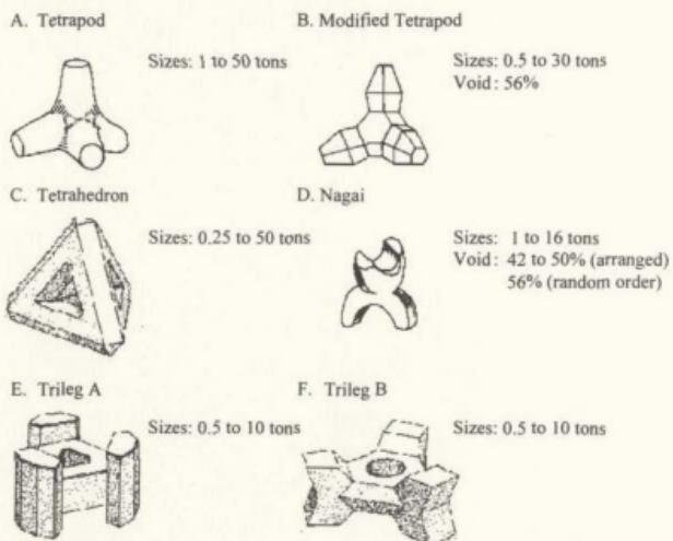
Figure 1.1. Manufactured Concrete Breakwater Blocks (Mottet, 1985)
