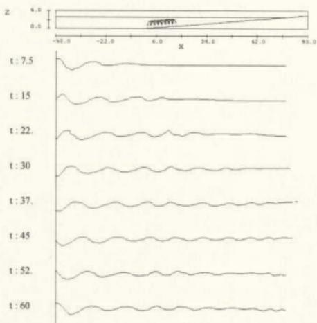
Figure 5.11 Wave Profile with Twenty-four Reefs, T: 3.5 sec
