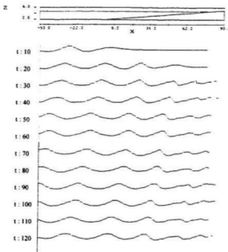
**Figure 4.6. Water Surface Profile without Reefs**
