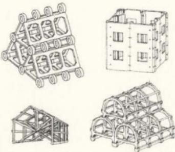
E. Fish habitat, Prefabricated Ferroconcrete
