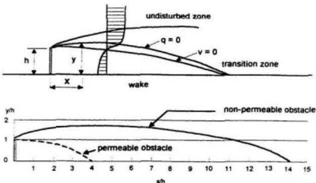
Figure 2.4. Current Shadow behind A Two-dimensional Obstacle
