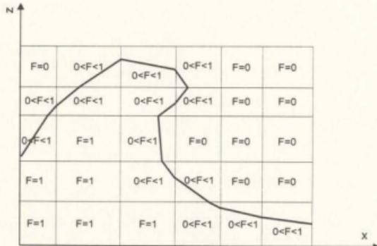
Figure 3.3 Typical Free Surface Cells
