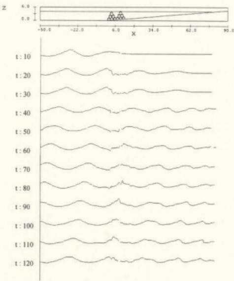
Figure 4.11 Water Surface Profile with Twelve Reefs
