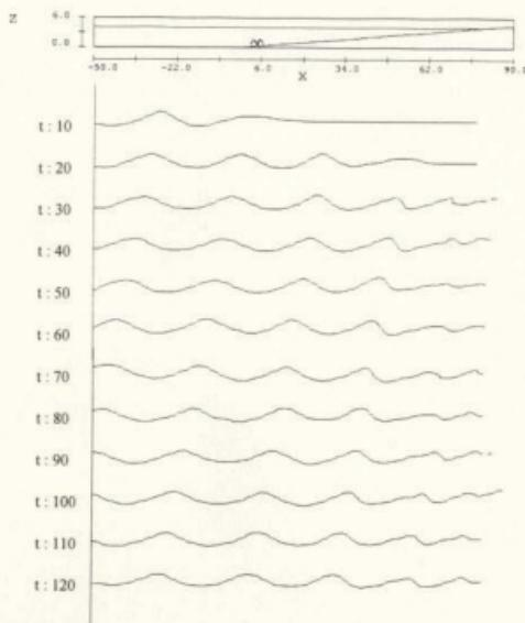
Figure 4.8. Water Surface Profile with Two Reefs
