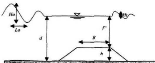
Figure 2.13 Geometry of Artificial Reefs
