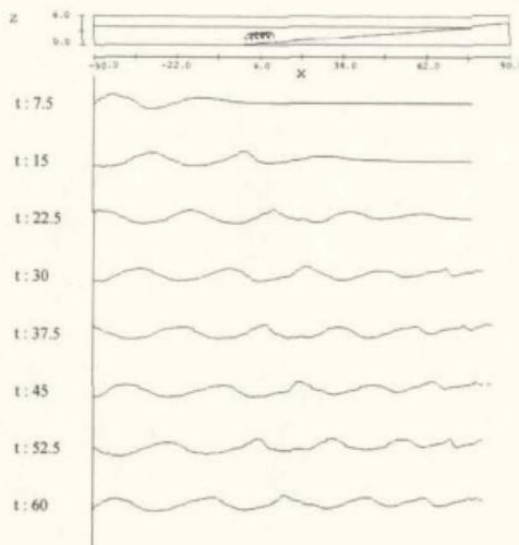
Figure 5.6. Wave Profile with Fifteen Reefs, T: 5.0 sec
