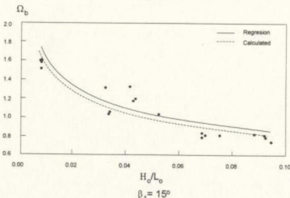
Figure 2.15 Breaker Height as A Function of Deepwater Steepness
