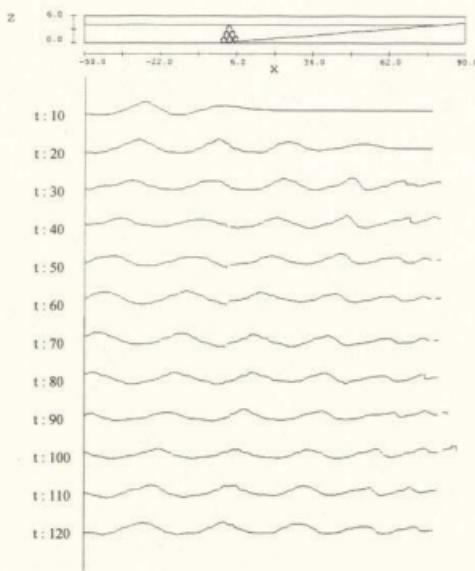
Figure 4.10. Water Surface Profile with Six Reefs
