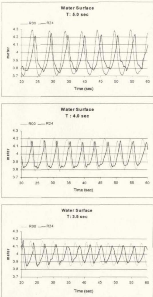
Figure 5.13. Surface Wave History for Three Different Periods at  $x: +18.0\text{m}$
