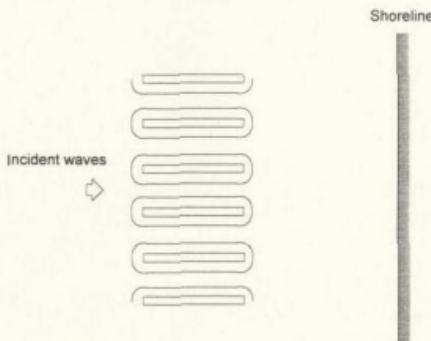
Figure 2.18 Longitudinal Artificial Reefs
