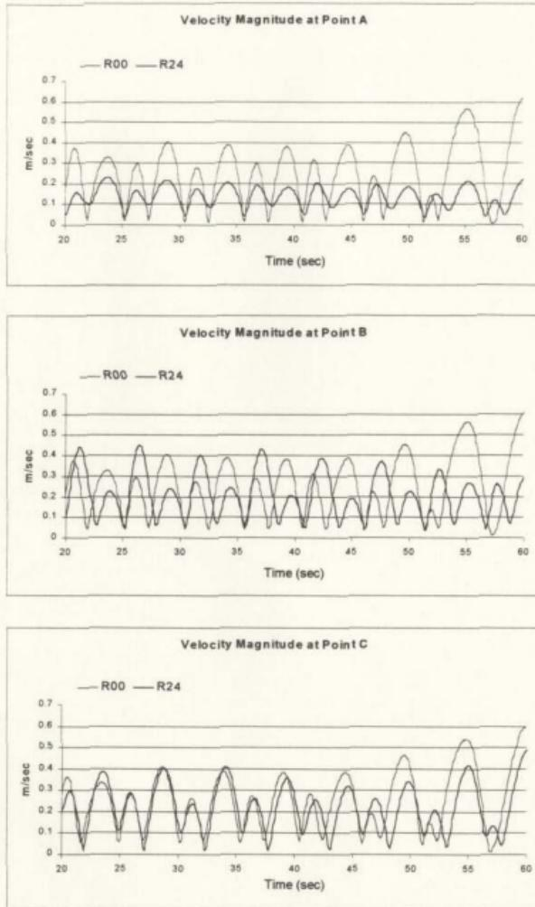
Figure 5.24 Velocity Magnitude Time Series for Twenty-four Reefs at Points A, B, and C
