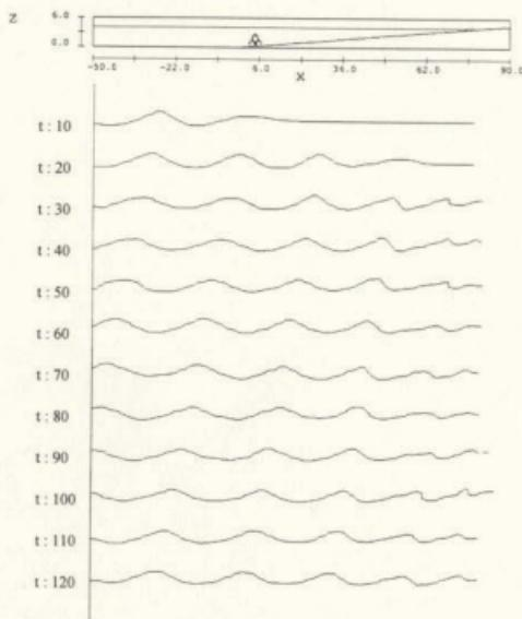
Figure 4.9 Water Surface Profile with Three Reefs
