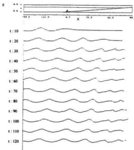
**Figure 4.7. Water Surface Profile with One Reef**
