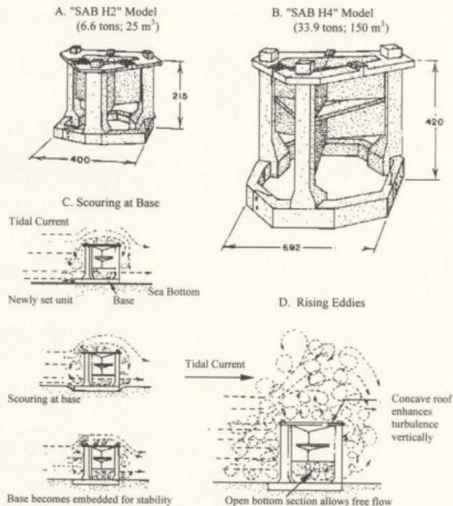
Figure 1.2 SAB Chamber Structures (Mottet, 1985)
