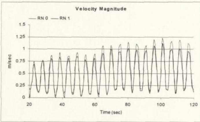
Figure 4.12 Water Surface Profile and Surface Velocity Magnitude Time Series for One Reef at  $x:+15.0\text{m}$
