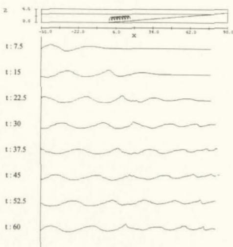
Figure 5.7. Wave Profile with Twenty-four Reefs, T: 5.0 sec
