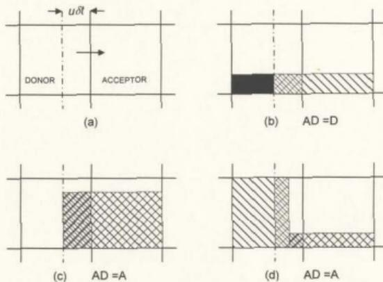
Figure 3.6 Examples of Free Surface Shapes used in The Advection of  $F$ .
