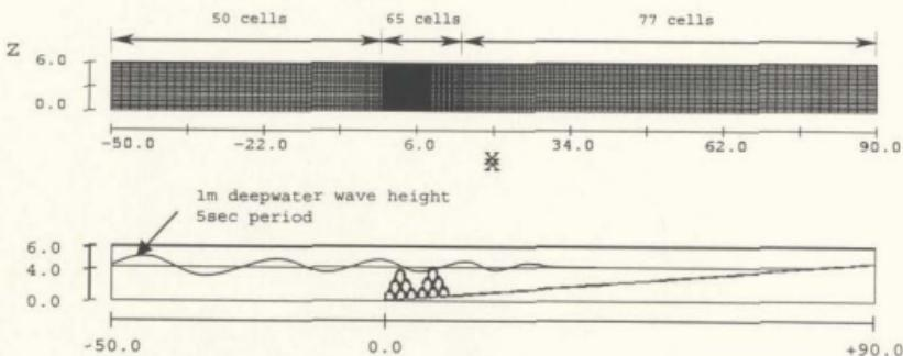
Figure 4.1. Typical Reef and Applied Grids
