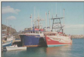
PLATE 5.1: THE 65' VESSELS "EASTERN PRINCESS" ON RIGHT BUILT IN 1980 AND "ATLANTIC SEA CLIPPER" ON LEFT BUILT IN 1990. NOTE PARAVANES IN UPRIGHT POSITION ON BOTH VESSELS.
