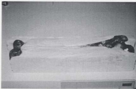
Figure 4.7 - Femur embedded in plaster in scan / load orientation. The sides of the plaster block are parallel to the load axis.
