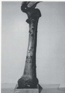
Figure 4.5 - Femur shown in four orientations with strain gages attached.
