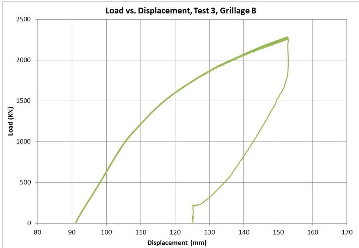
Figure 2-16: Load vs. displacement, test 3, grillage B
