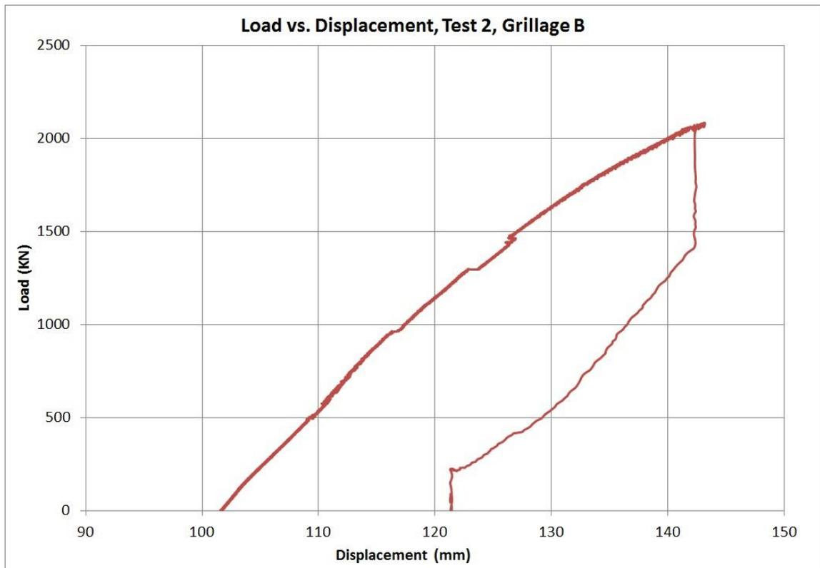
**Figure 2-15: Load vs. deformation, test 2, grillage B**
