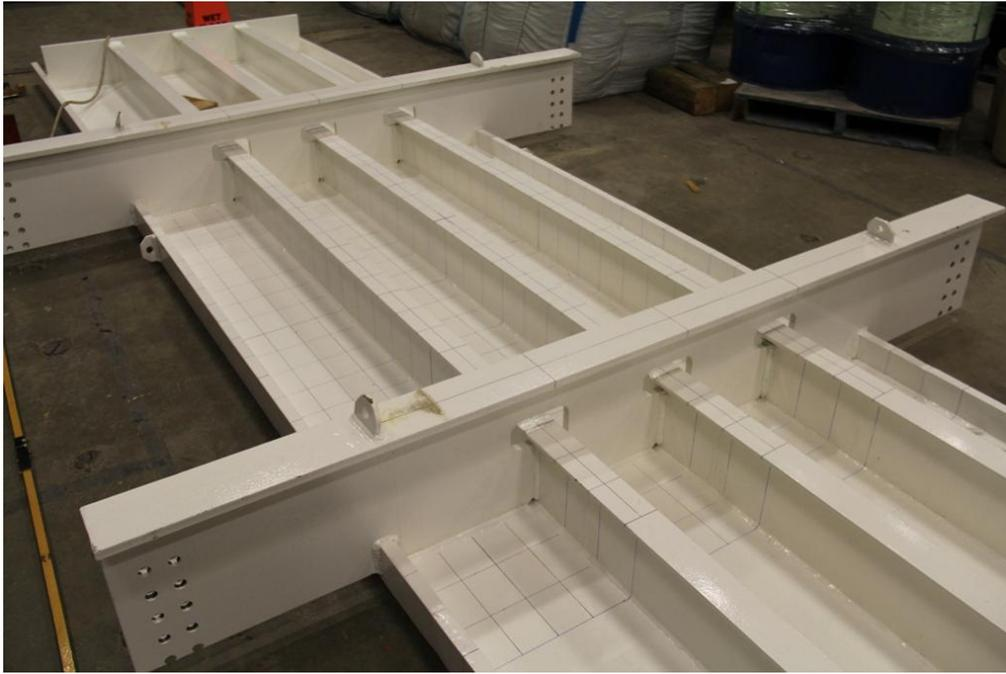
**Figure 2-3: Undeformed grillage**
