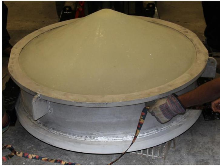
**Figure 2-2: Prepared ice cone**
