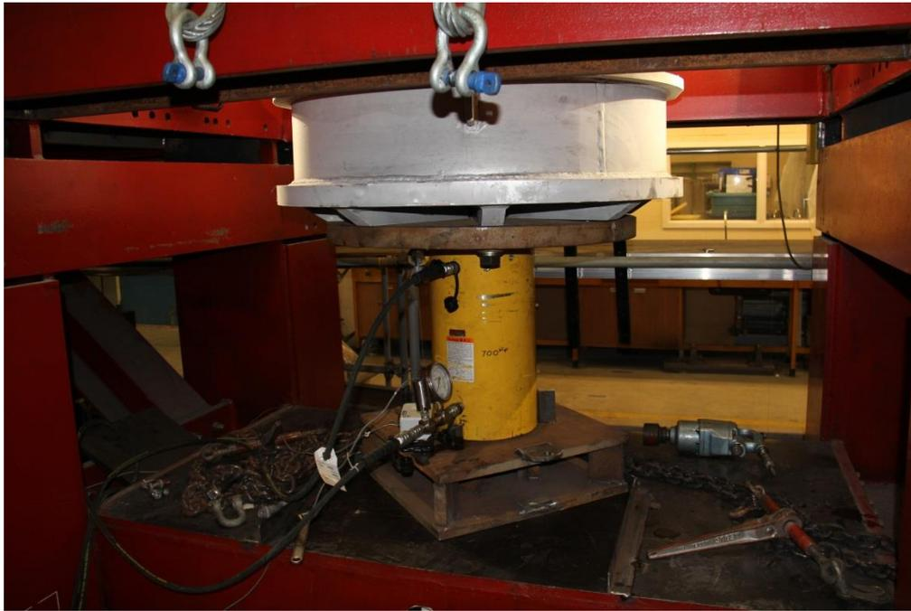
**Figure 2-5: Ice cone mounted on hydraulic ram, ready for experiment**
