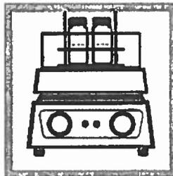
**11. Place the assembly in the hot water bath when the water is boiling rapidly.** Do not allow the water to rise above the white "diamond" near the top of the sample cells.
