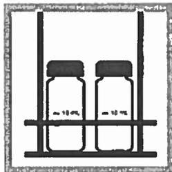
**10. Place the sample cells in the cell holder assembly.**
