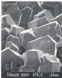
Fig. 2.16 a) and b) Backscattered electron photographs of calcium tartrate crystals from Scherzinger's Pinot Noir, 1997, at magnification of X70(a) and X150(b). Crystals were removed from wine by filtration, coated with carbon and imaged using a scanning electron microscope (SEM) with a working distance of 23 \mu m, a takeoff angle of 30°, and an accelerating voltage of 20kV.
