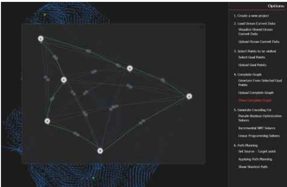
Figure 5: Complete graph generated from selected goal points (Figure 1) with an optimal sequence highlighted.
