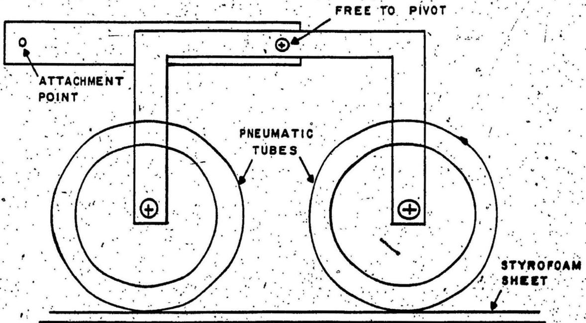
FIGURE 22 SINGLE AND TWO TIRE MODELS
