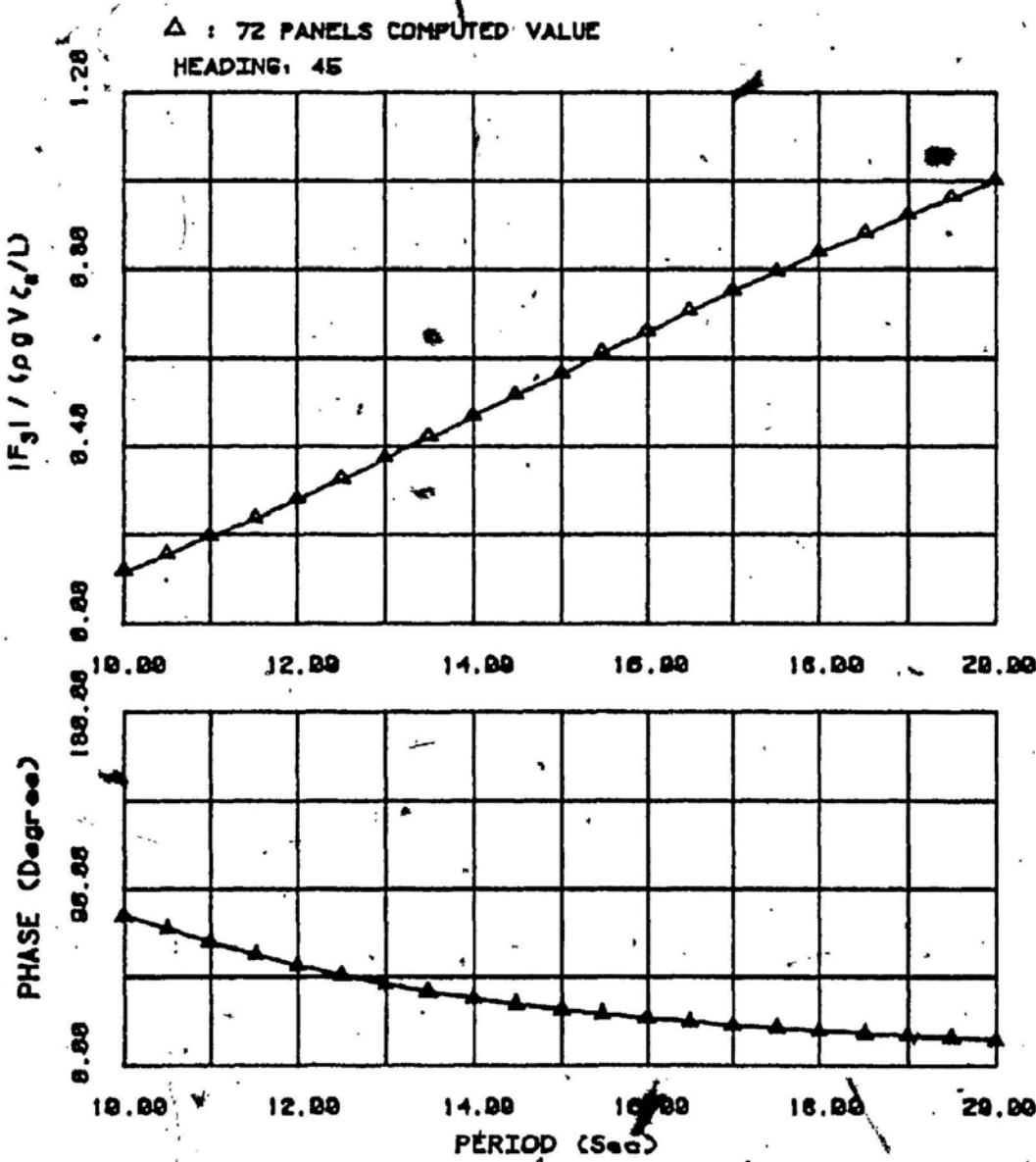
Figure (18.b) Heave exciting force and phase for rectangular box
