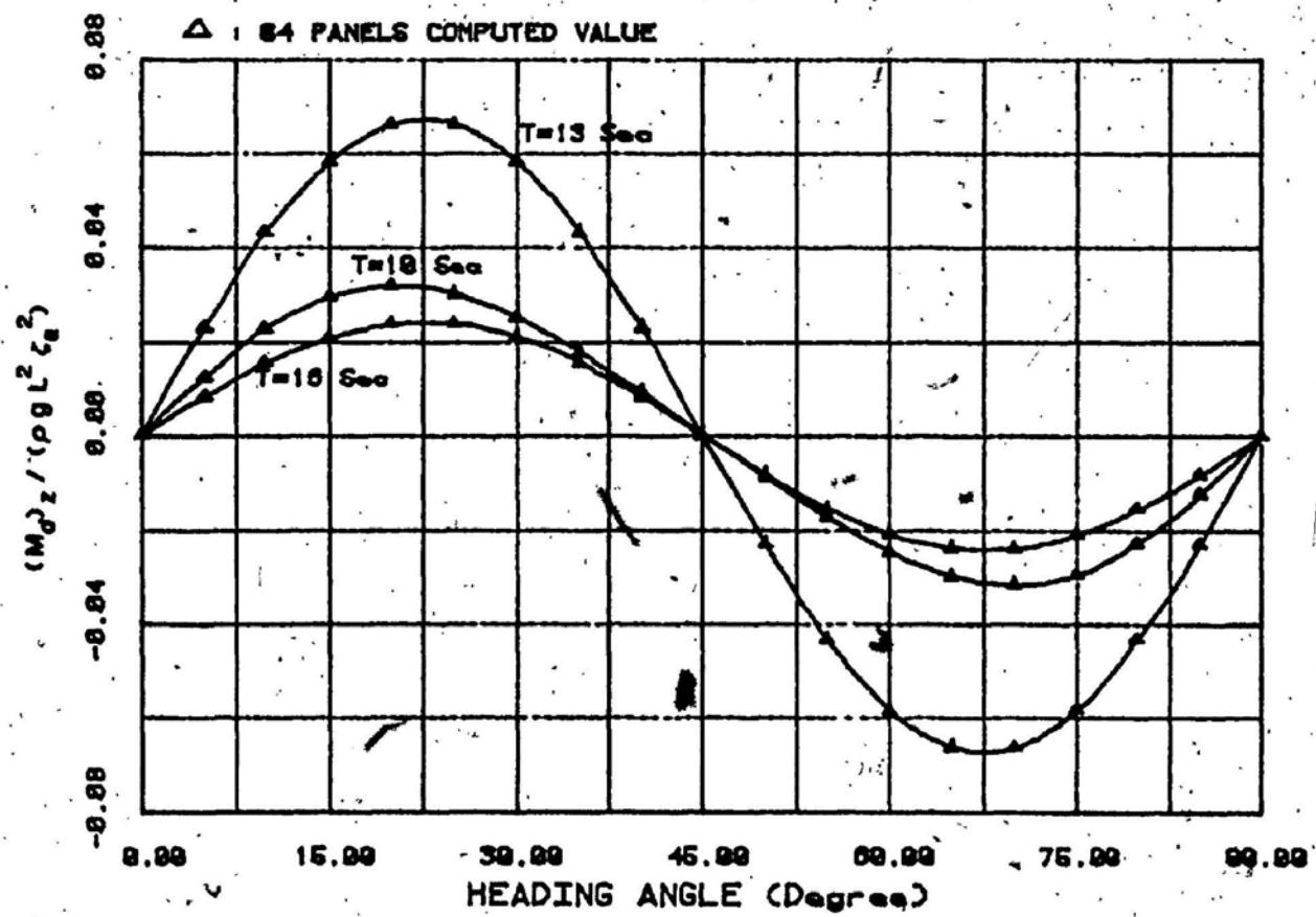
Figure (22) Vertical Drift moment for rectangular box
