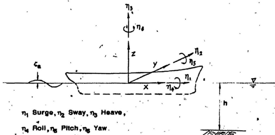
Figure (1) Coordinate system and sign convention for translatory and angular displacements
