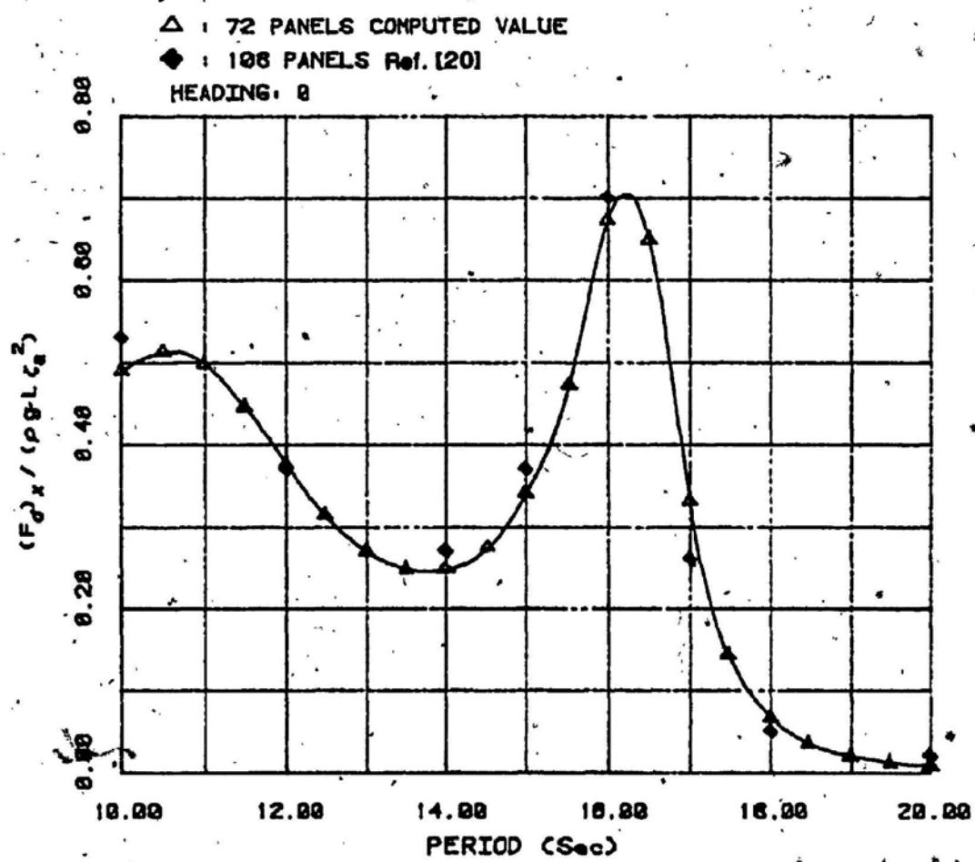
Figure (20.a) Drift force in x-component for rectangular box
