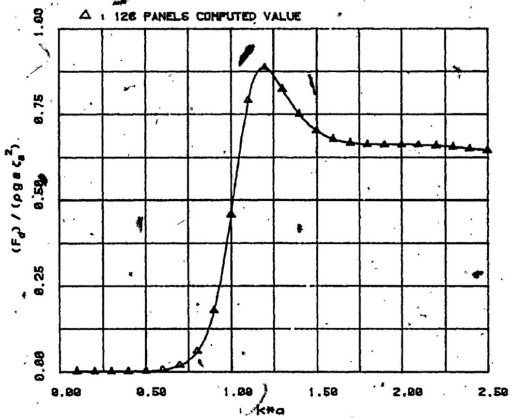
Figure (8) Drift force for a hemisphere ( $h/a = 10$ )
