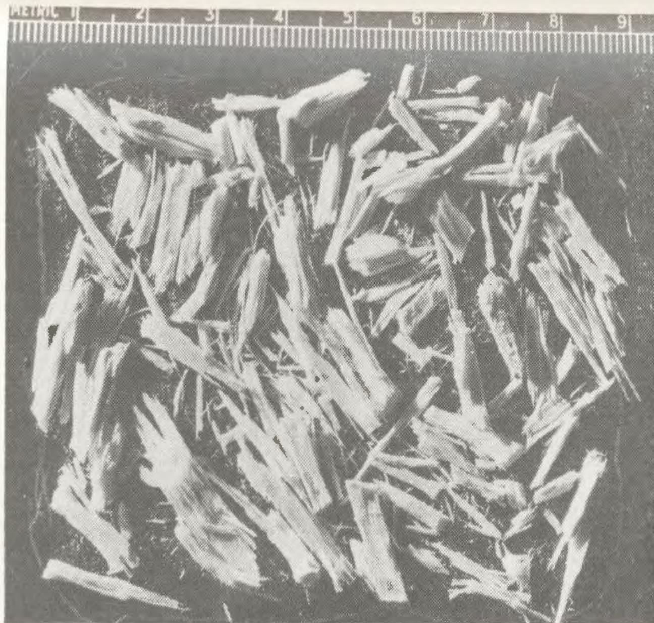
Fig. 41. Material sampled after passing through the breaker bar section alone. The fragments are seen to be quite uniform and the major axis of each is in the grain direction.
