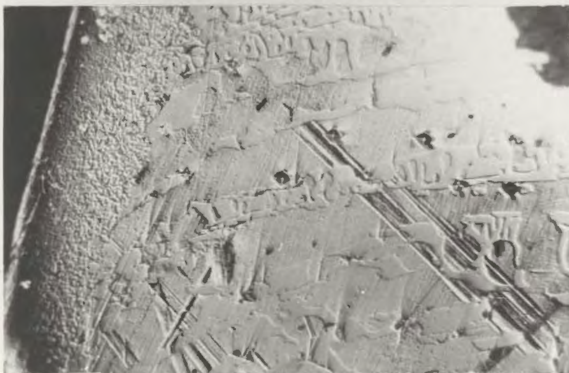
Fig. 67. Sample Site R-1 I-8 showing microhardness marks - 300X, Normanski interference, etched.
