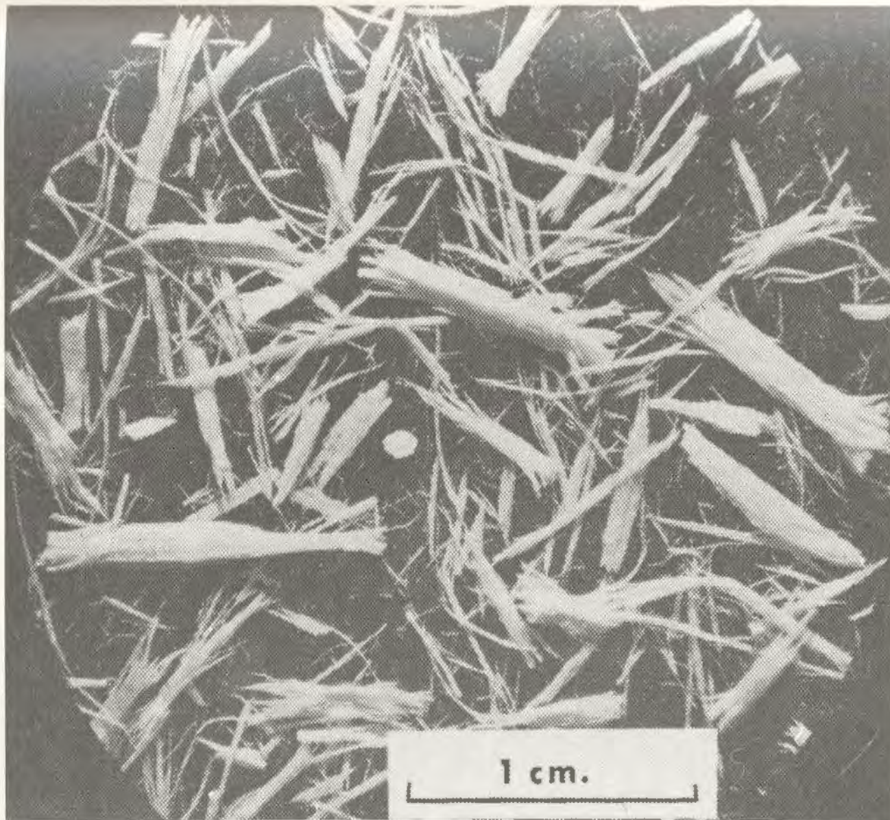
Fig. 43. Material sampled after moving a radial distance of 2.5 in. from the breaker bar section. Note the cylindrical aspect of some of the larger fragments.
