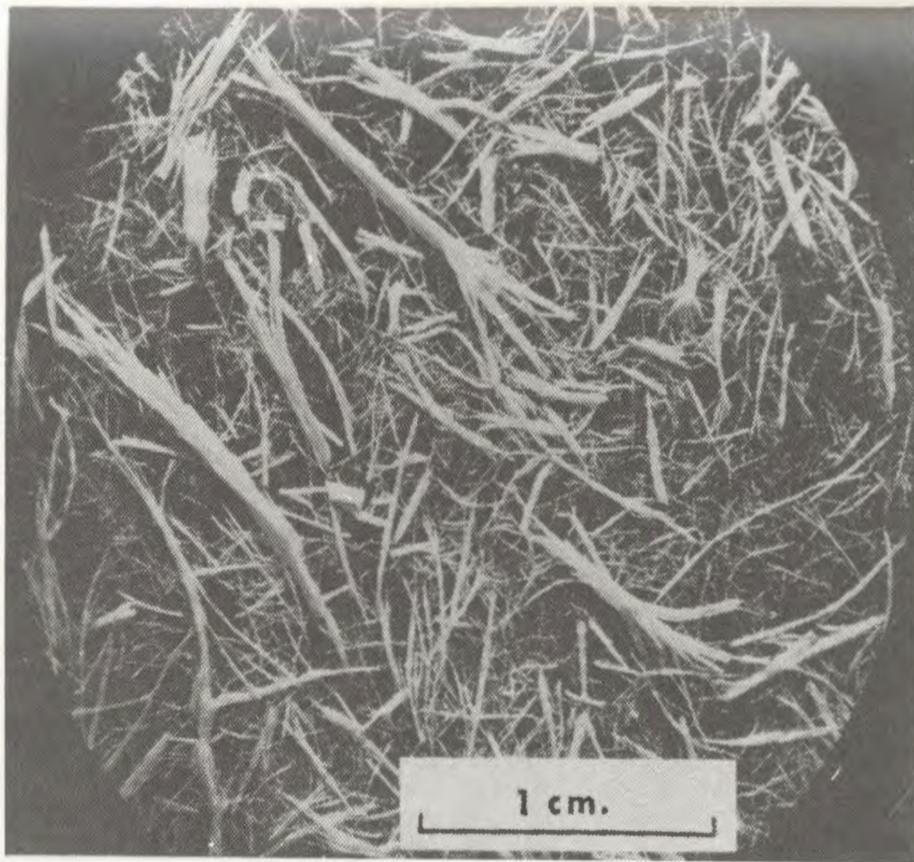
Fig. 44. Material sampled after moving a radial distance of 4.0 in. from the breaker bar section. Note the broomed ends of many cylindrical fragments.
