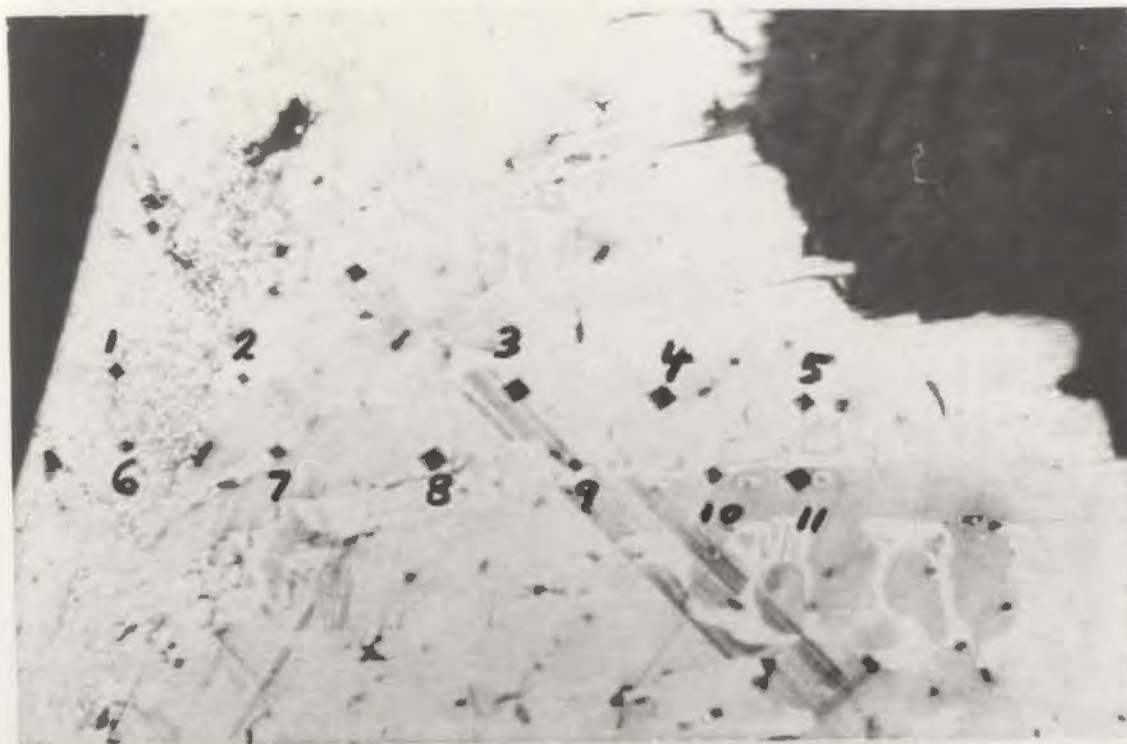
Fig. 66. Sample Site R-1 I-8 showing microhardness marks - 300X, etched.
