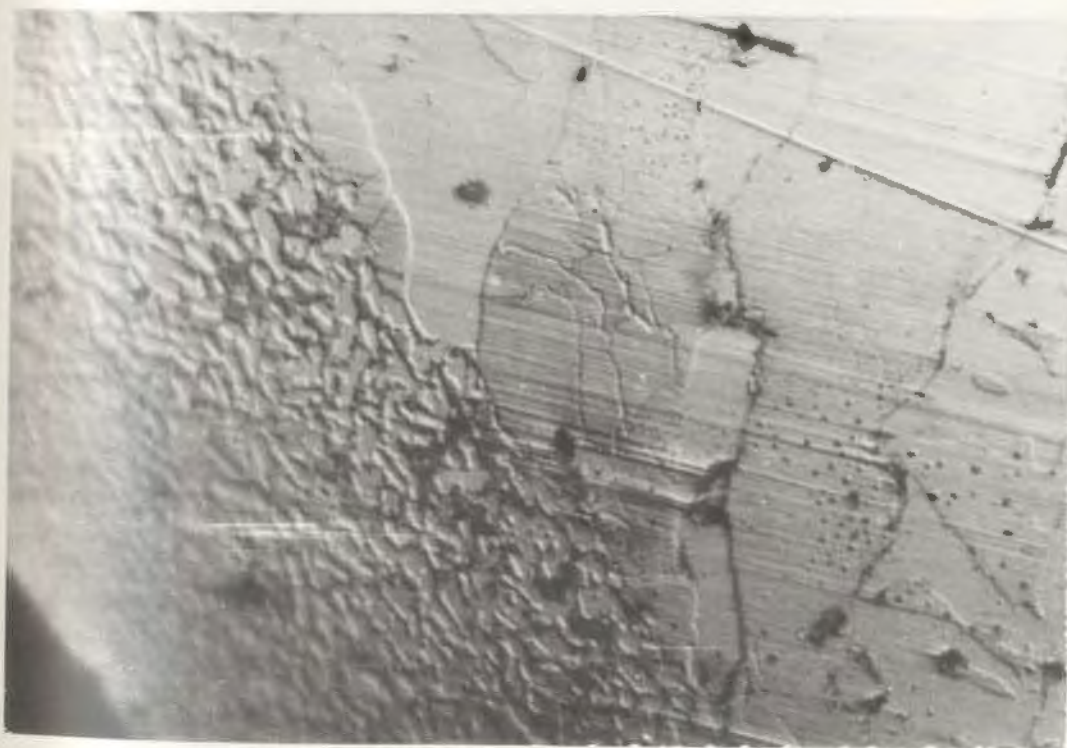
Fig. 65. Sample Site R-1 I-8 - 1000X, Normanski interference, end of layer 3, layer 4 in focus, etched.
